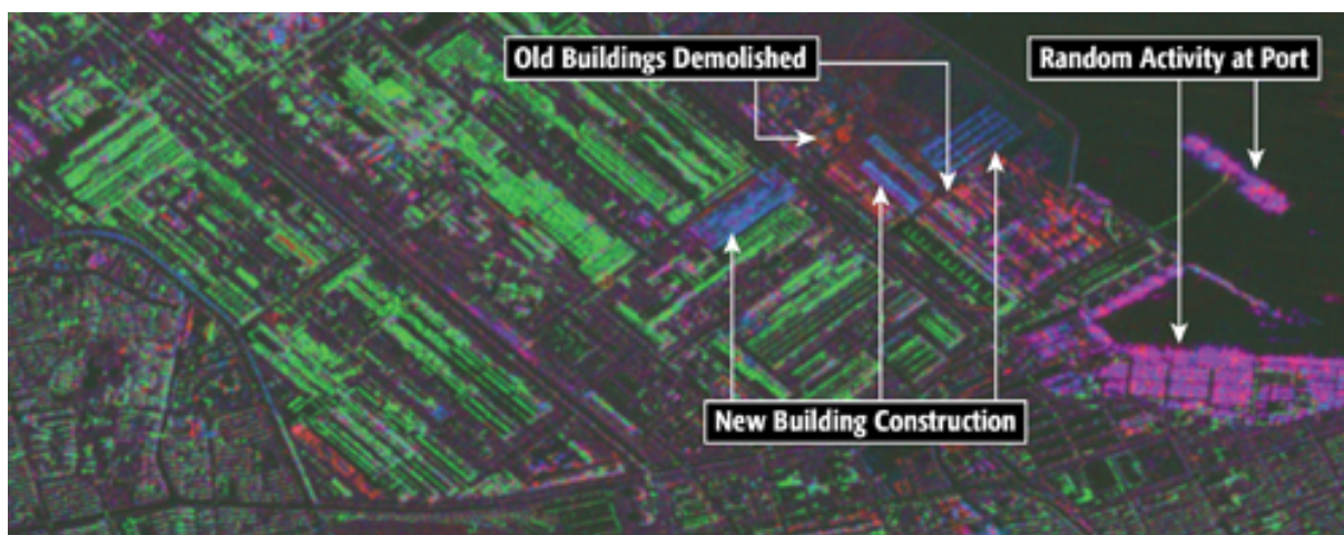
Figure 1 - Radar change detection at a port; CD identifies new buildings (blue) and buildings torn down (red) 30
