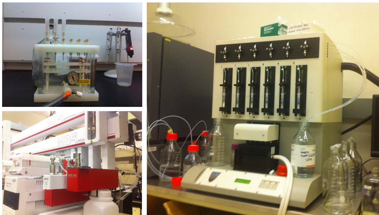
Figure 1-2. SPE equipment in the laboratory. Clockwise from upper left: Vacuum manifold (Thermo Fisher Scientific, Waltham, Massachusetts), automated large-volume SPE extraction instrument (Dionex, Bannockburn, Illinois), and integrated SPE sample preparation on a gas chromatograph-mass spectrometer (GC-MS; Gerstel GmbH & Co.KG, Mülheim an der Ruhr, Germany).
