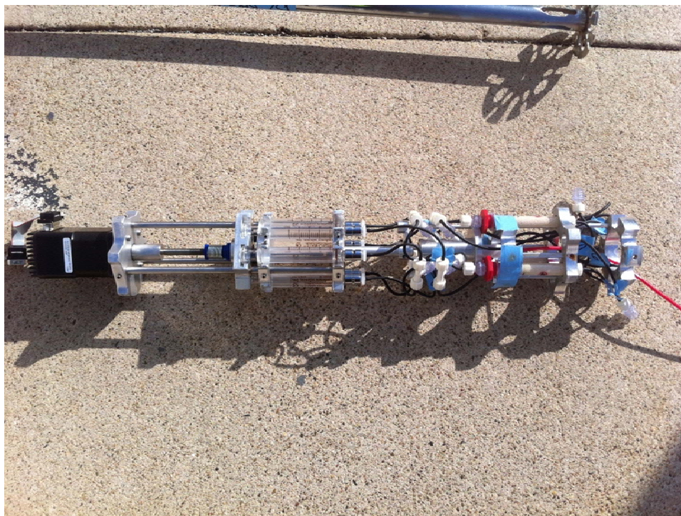
Figure 5-12. Field-prepared IS2 sampler with reciprocating syringe pump.
