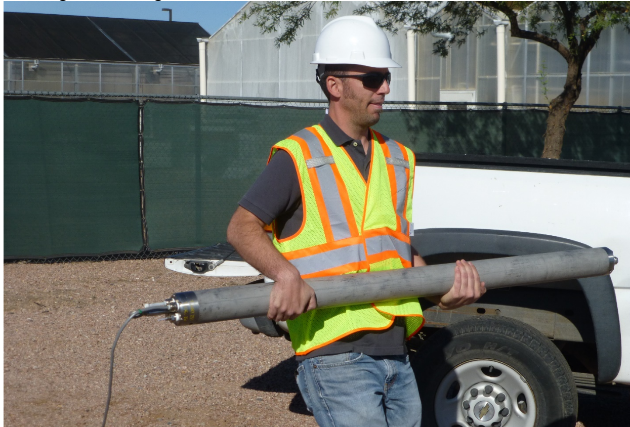
Figure 5-8. IS2 sampler with peristaltic pump in its watertight shell. Ports in the shell provide fluid inlets, gas pressure relief, and electrical connections.
