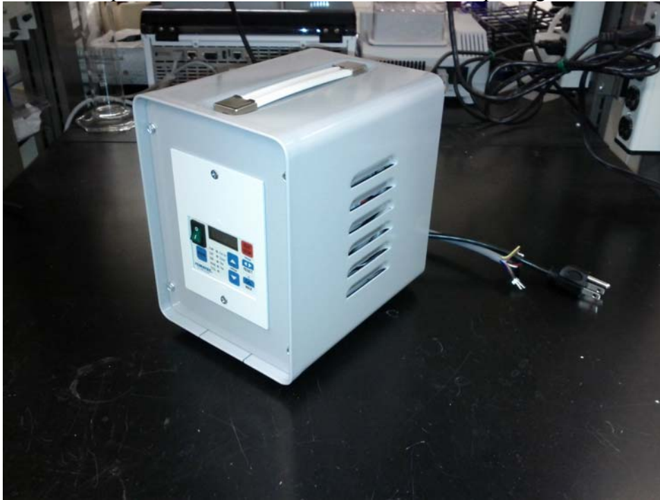
Figure 5-9. IS2 peristaltic pump control unit. The control unit powers and controls the peristaltic pump in the sampler.
