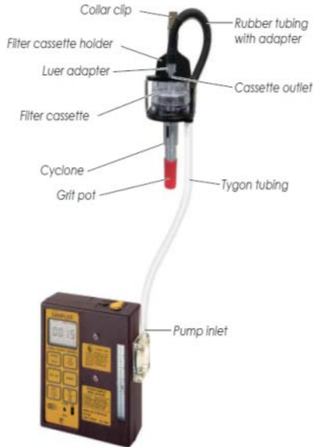
Filter and Cyclone Sample Train Assembly
