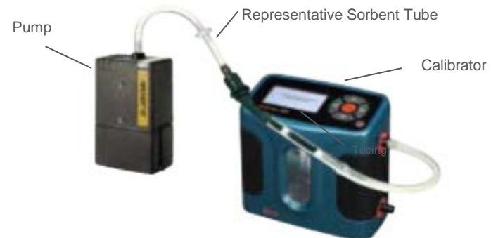
Calibration train with tube in low flow holder
