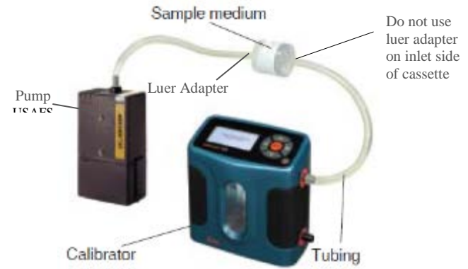
Calibration train with filter cassette
