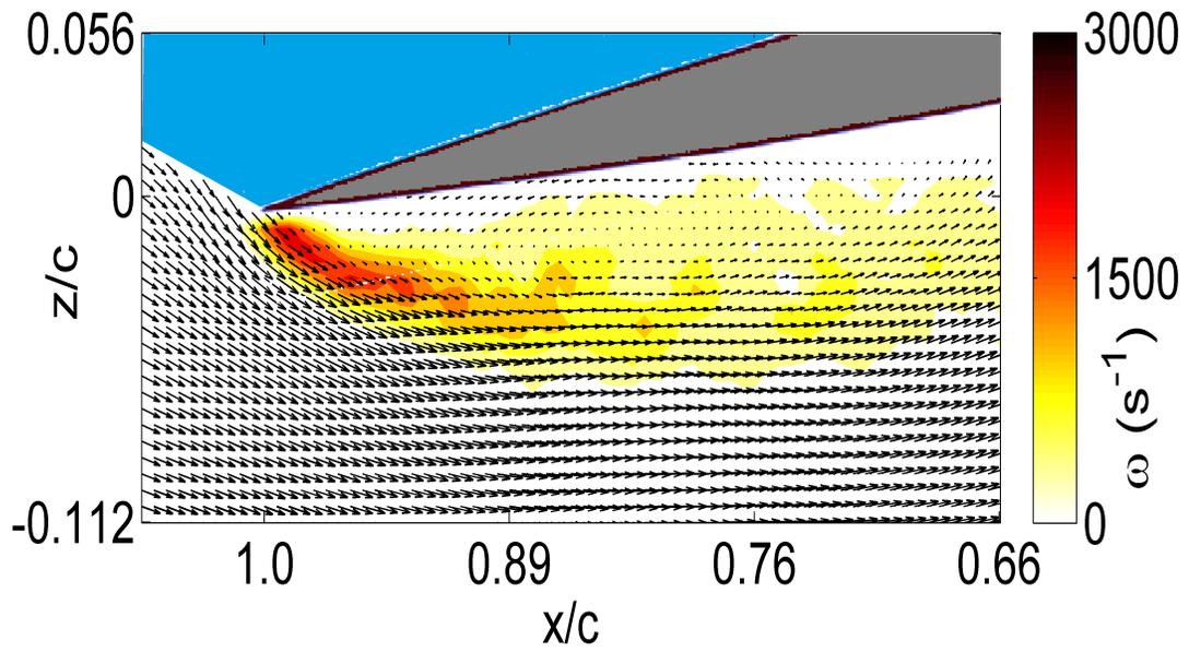
**Figure 103:** Velocity field on a static wing showing the existence of a vortex at  $\psi = 30^\circ$ ,  $\alpha = 192^\circ$ ,  $Re = 0.63 \times 10^5$
