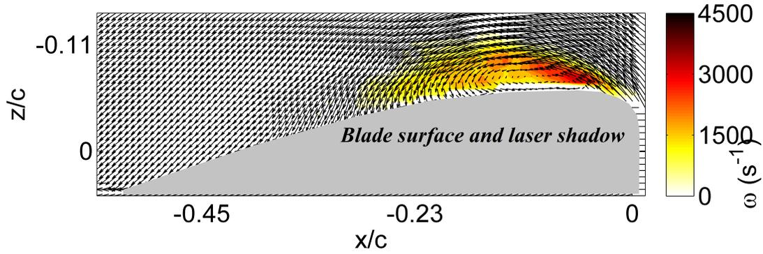
**Figure 38:** Velocity field at  $\psi = 315^\circ$ ,  $r/R = 0.6$ ,  $\mu = 0.4$
