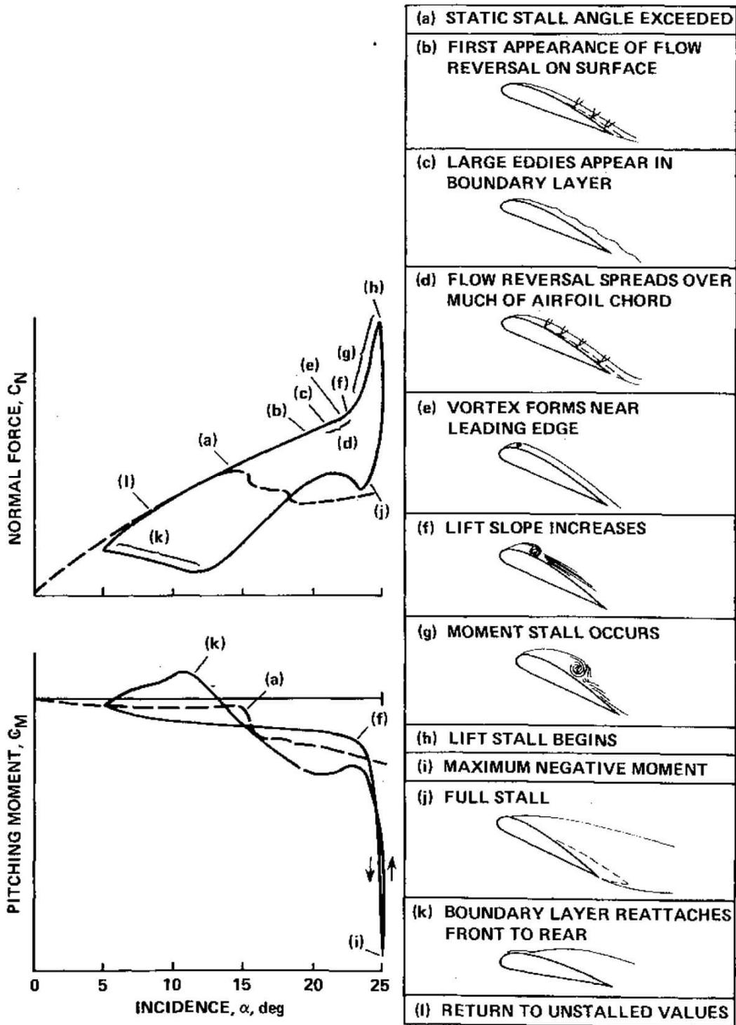
Figure 2: Events of dynamic stall on a NACA 0012 airfoil adopted from Carr [13].
