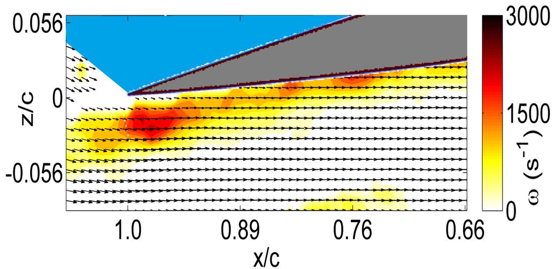
**Figure 107:** Velocity field on a rotating wing overlaid on vorticity contours at  $\psi = 240^\circ$ ,  $\mu = 0.8$  and  $\Omega = 20.93 \text{ rad/s}$  which yields  $\alpha = 192^\circ$  and  $Re = 0.63 \times 10^5$  at  $r/R = 0.5$
