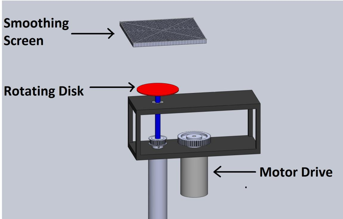
**Figure 82:** Drawing of the rotating disk setup
