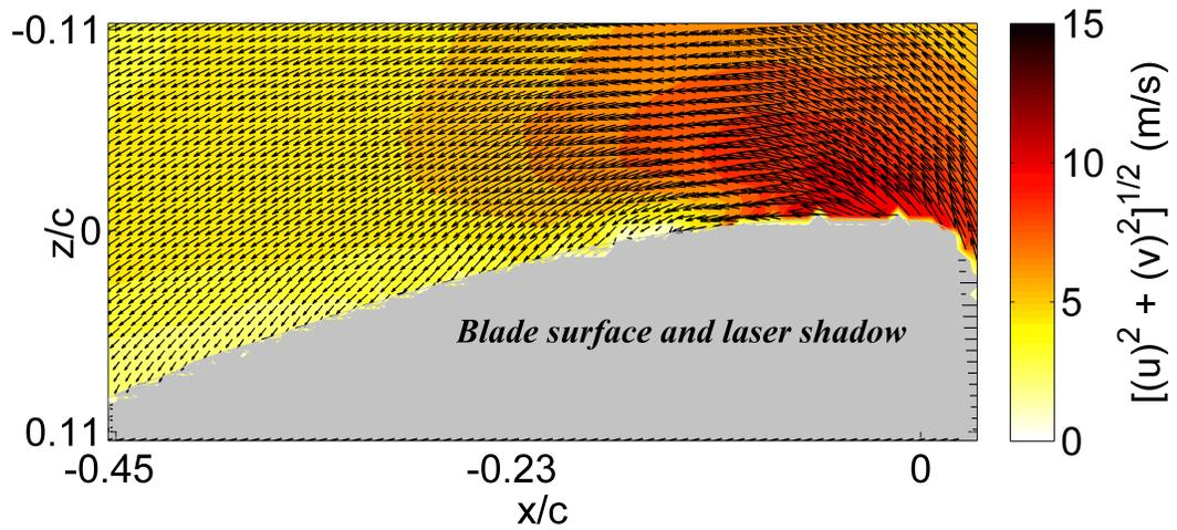
**Figure 20:** Velocity field at  $\psi = 230^\circ$ ,  $r/R = 0.6$ ,  $\mu = 0.35$
