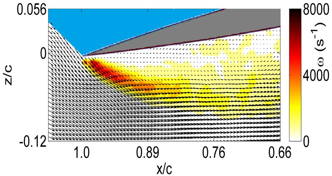
**Figure 104:** Velocity field on a static wing showing the existence of a vortex at  $\psi = 30^\circ$ ,  $\alpha = 195^\circ$ ,  $Re = 1.7 \times 10^5$
