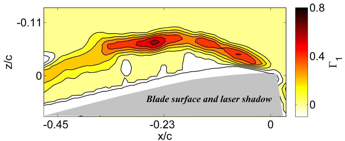
**Figure 27:** NAM plot at  $\psi = 252.6^\circ$ ,  $r/R = 0.6$ ,  $\mu = 0.4$
