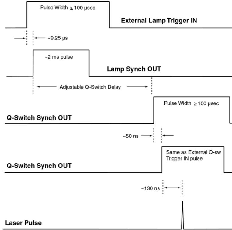
**Figure 7:** Timing diagram for a PIV experiment.
