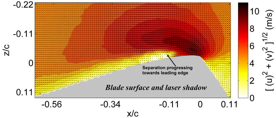
**Figure 15:** Velocity field at  $\psi = 220^\circ$ ,  $r/R = 0.5$ ,  $\mu = 0.4$  showing the progression of separation at trailing edge at higher advance ratio
