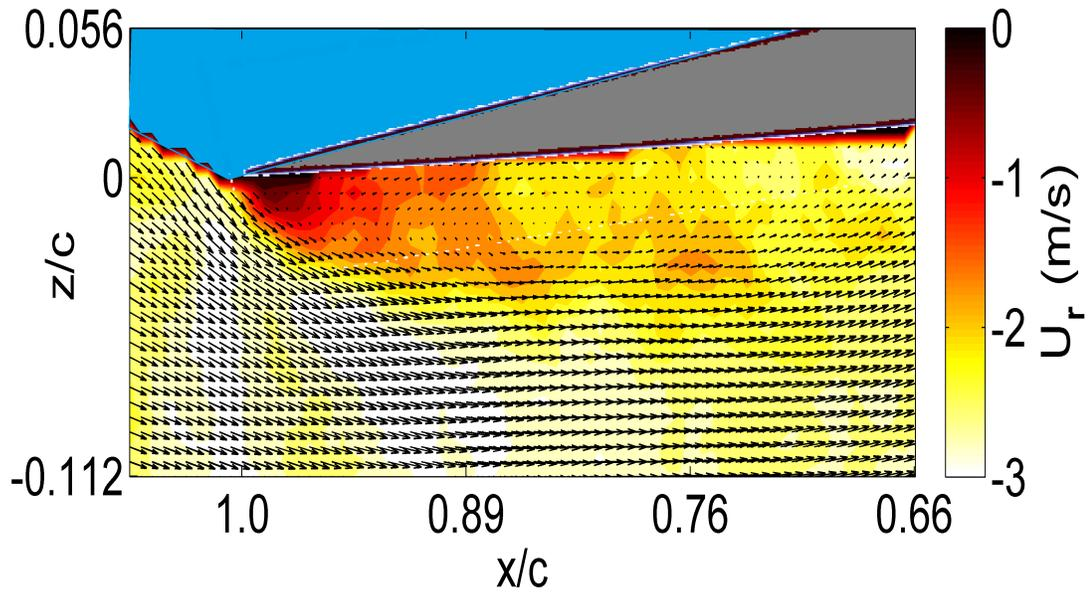
**Figure 105:** Velocity field on a static wing overlaid on the radial (spanwise) component of velocity at  $\psi = 30^\circ$ ,  $\alpha = 192^\circ$ ,  $Re = 0.63 \times 10^5$
