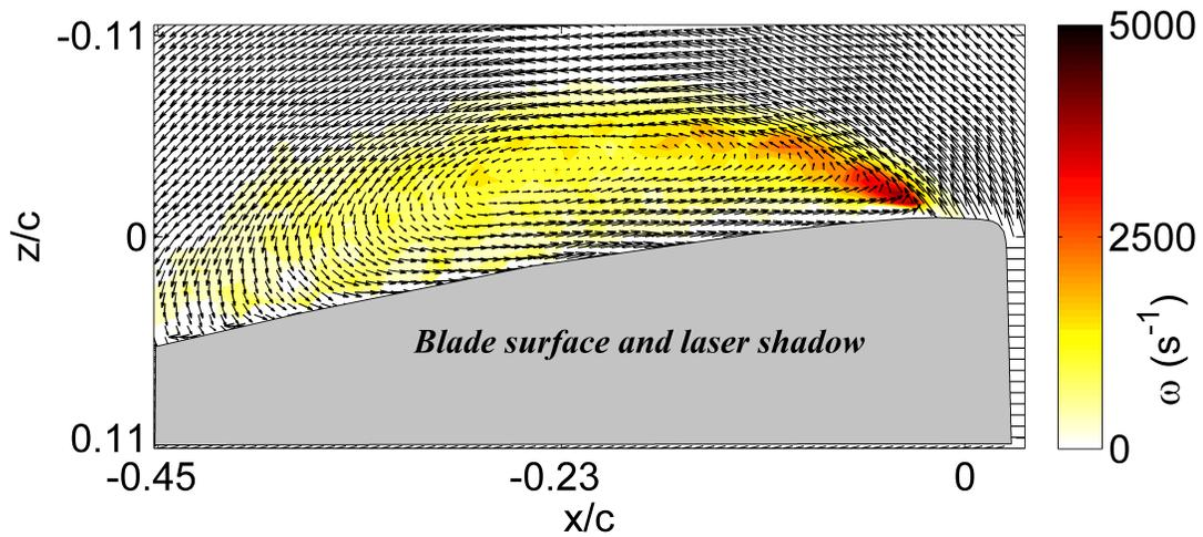
**Figure 23:** Velocity field at  $\psi = 235^\circ$ ,  $r/R = 0.6$ ,  $\mu = 0.4$
