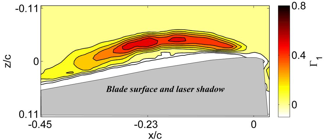
**Figure 25:** NAM plot at  $\psi = 235^\circ$ ,  $r/R = 0.6$ ,  $\mu = 0.4$
