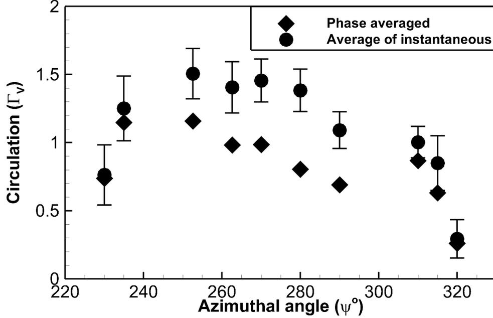
**Figure 49:** Variation of circulation of the flow over the upper surface of the rotating blade with azimuthal angle computed using phase averaged and instantaneous velocity fields at  $r/R = 0.6$  and  $\mu = 0.4$
