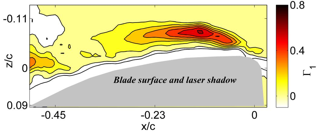
**Figure 35:** NAM plot at  $\psi = 290^\circ$ ,  $r/R = 0.6$ ,  $\mu = 0.4$
