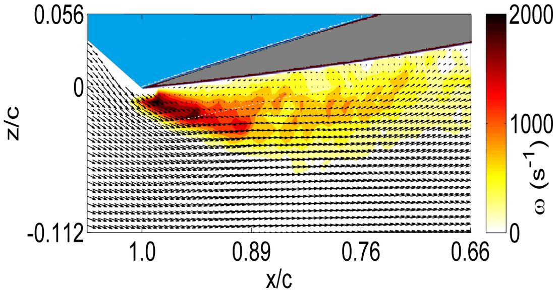
**Figure 102:** Velocity field on a static wing showing the existence of a vortex at  $\psi = 30^\circ$ ,  $\alpha = 191.2^\circ$ ,  $Re = 0.63 \times 10^5$
