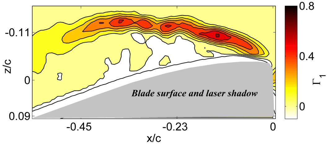
**Figure 31:** NAM plot at  $\psi = 270^\circ$ ,  $r/R = 0.6$ ,  $\mu = 0.4$
