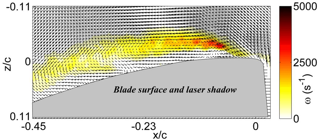
**Figure 22:** Velocity field at  $\psi = 235^\circ$ ,  $r/R = 0.6$ ,  $\mu = 0.35$
