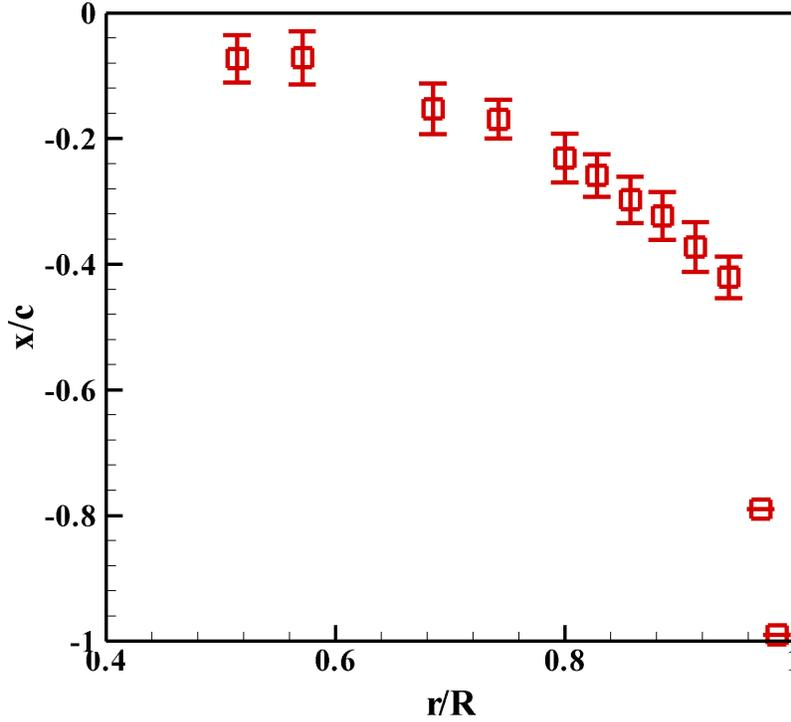
**Figure 60:** Radial variation of the phase-averaged separation line, with error bars showing standard deviation, the  $x/c = 0$  location is the blade leading edge, while  $x/c = -1$  is the blade trailing edge
