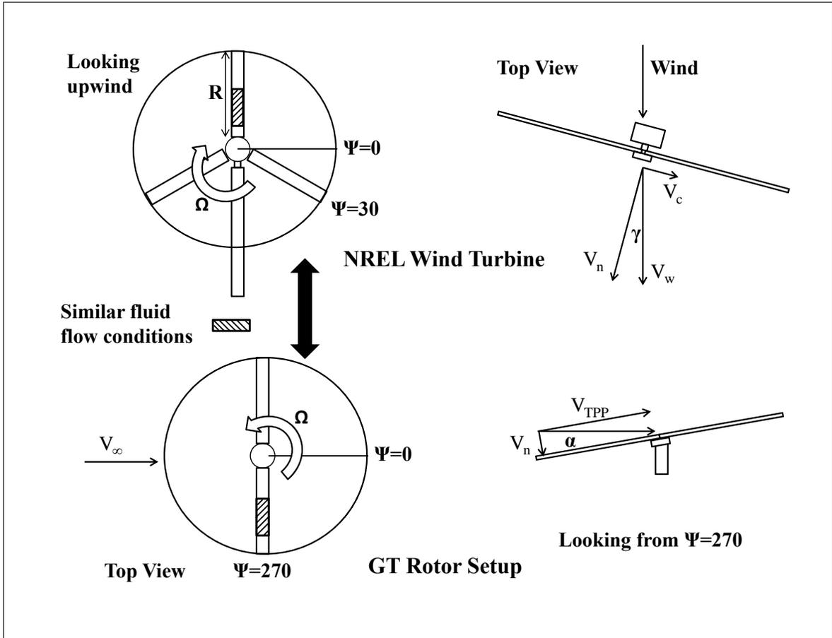
**Figure 113:** Schematic representation of similar fluid flow conditions.
