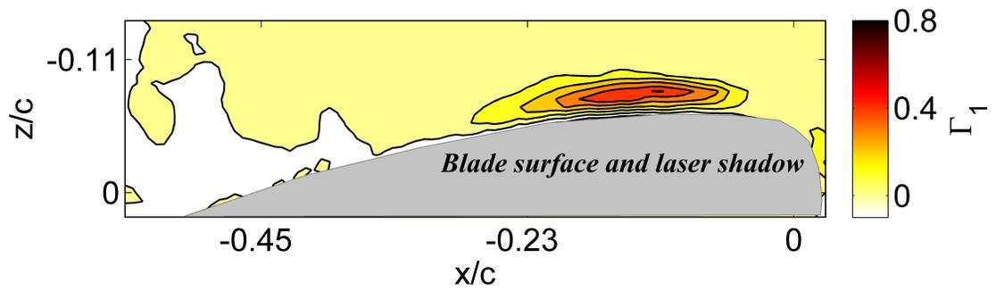
Figure 39: NAM plot at  $\psi = 315^\circ$ ,  $r/R = 0.6$ ,  $\mu = 0.4$
