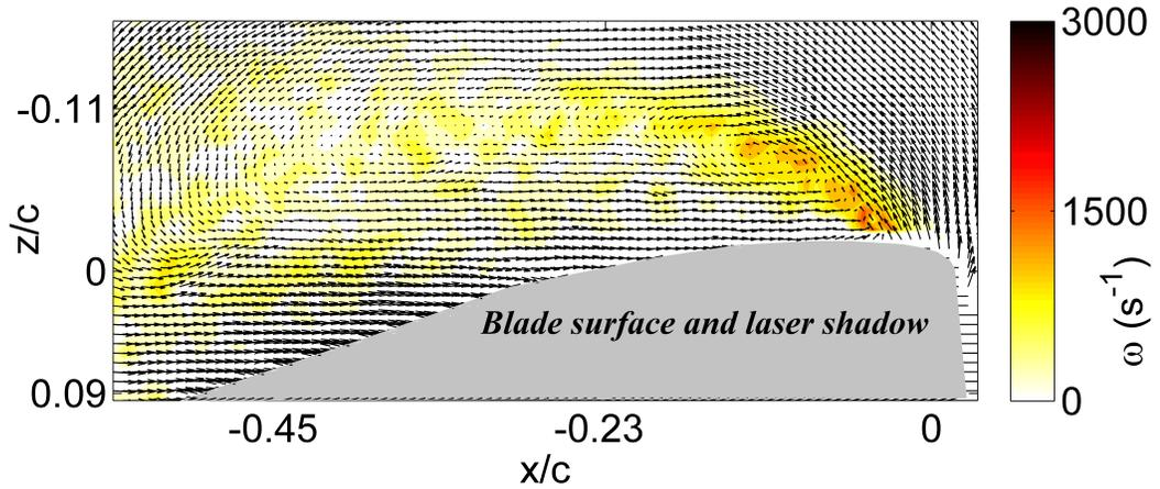
**Figure 28:** Velocity field at  $\psi = 262.6^\circ$ ,  $r/R = 0.6$ ,  $\mu = 0.4$
