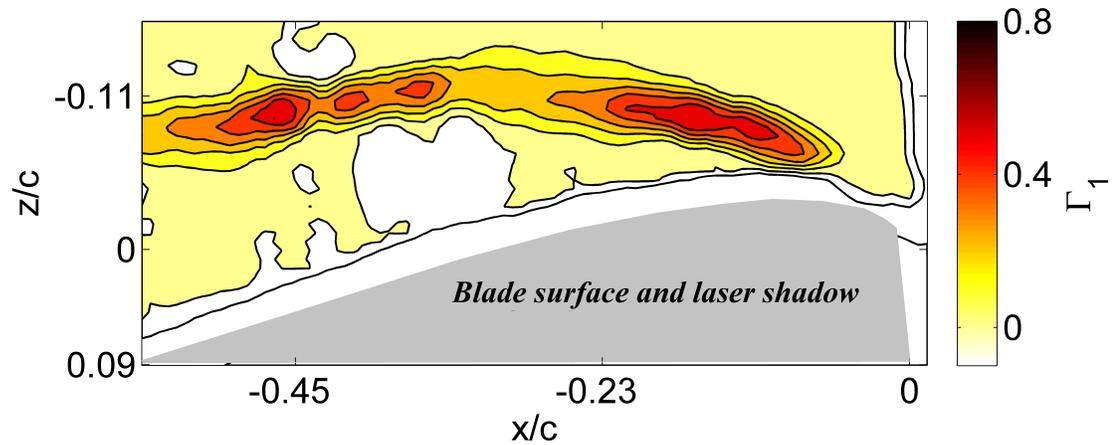
**Figure 33:** NAM plot at  $\psi = 280^\circ$ ,  $r/R = 0.6$ ,  $\mu = 0.4$
