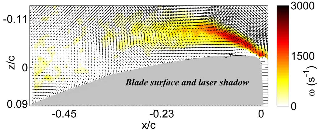
**Figure 34:** Velocity field at  $\psi = 290^\circ$ ,  $r/R = 0.6$ ,  $\mu = 0.4$
