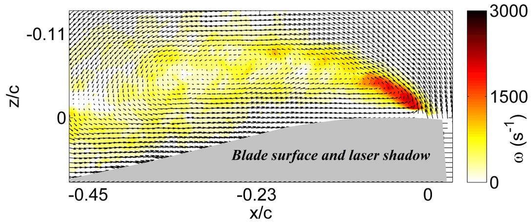
**Figure 26:** Velocity field at  $\psi = 252.6^\circ$ ,  $r/R = 0.6$ ,  $\mu = 0.4$
