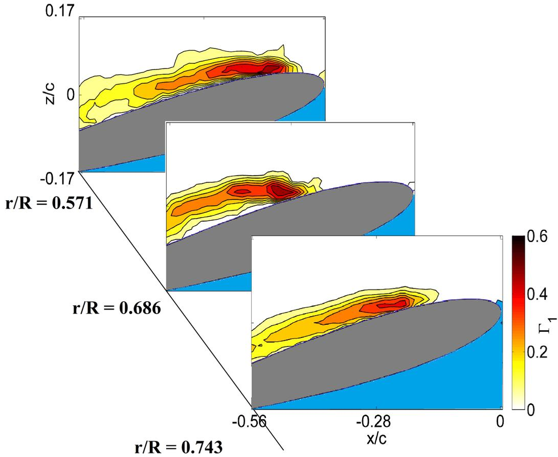
**Figure 57:** Illustration of the variation of the vortex at several radial locations
