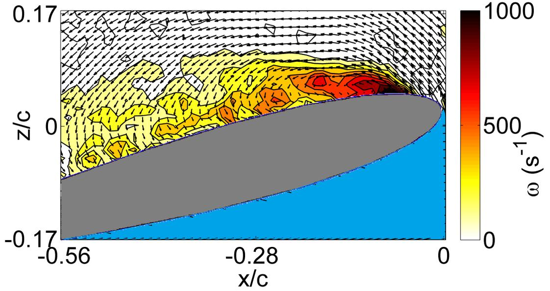
**Figure 51:** Velocity field at  $r/R = 0.514$ ,  $k = 0.54$ ,  $Re = 39,455$
