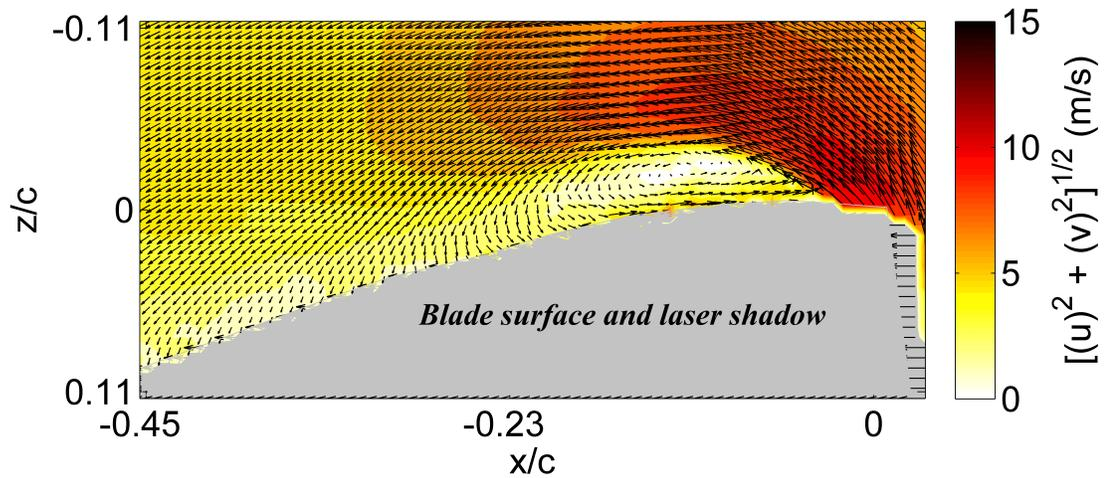
**Figure 21:** Velocity field at  $\psi = 230^\circ$ ,  $r/R = 0.6$ ,  $\mu = 0.4$
