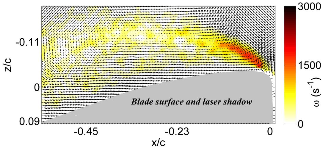
**Figure 30:** Velocity field at  $\psi = 270^\circ$ ,  $r/R = 0.6$ ,  $\mu = 0.4$
