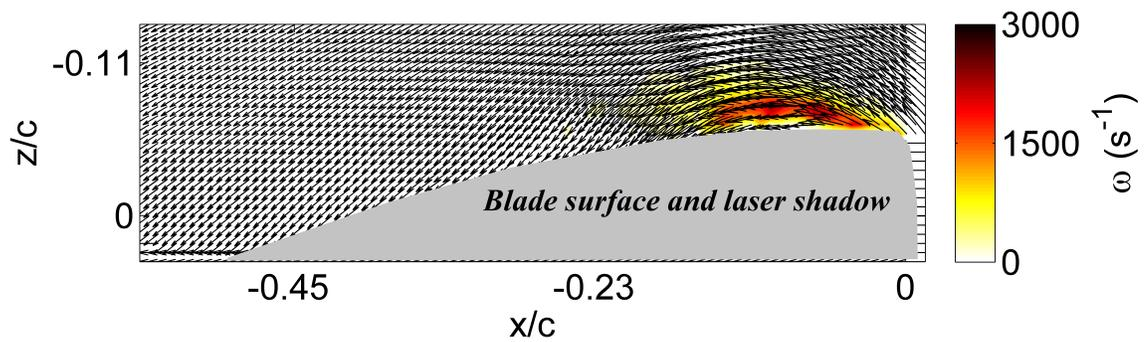
Figure 40: Velocity field at  $\psi = 320^\circ$ ,  $r/R = 0.6$ ,  $\mu = 0.4$
