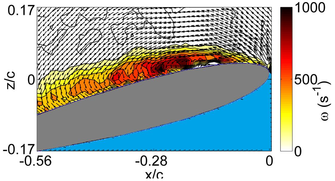
**Figure 52:** Velocity field at  $r/R = 0.743$ ,  $k = 0.24$ ,  $Re = 87,767$
