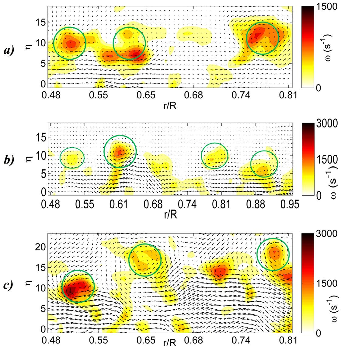
**Figure 92:** PIV velocity vector field illustrating a typical set of co-rotating vortices above the rotating disk at  $\alpha=8^\circ$  for a)  $\text{Re}=126$  and  $\mu = 1.39$ , b)  $\text{Re}=154$  and  $\mu = 0.92$  and c)  $\text{Re}=199$  and  $\mu = 0.55$
