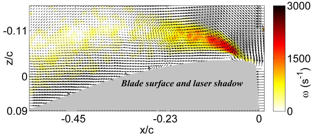
**Figure 32:** Velocity field at  $\psi = 280^\circ$ ,  $r/R = 0.6$ ,  $\mu = 0.4$
