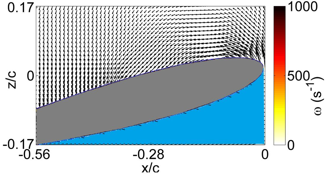
**Figure 53:** Velocity field at  $r/R = 0.971$ ,  $k = 0.16$ ,  $Re = 136,079$
