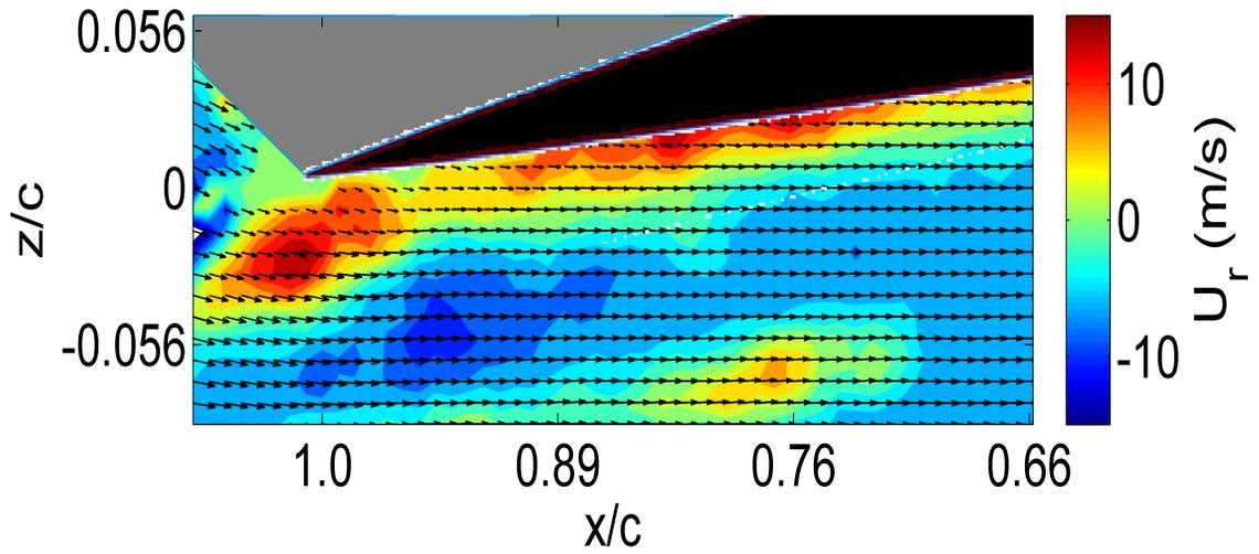
**Figure 106:** Velocity field on a rotating wing overlaid on the radial (spanwise) component of velocity at  $\psi = 240^\circ$ ,  $\mu = 0.8$  and  $\Omega = 20.93 \text{ rad/s}$  which yields  $\alpha = 192^\circ$  and  $Re = 0.63 \times 10^5$  at  $r/R = 0.5$
