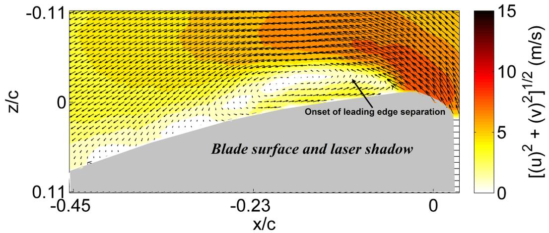
**Figure 18:** Velocity field at  $\psi = 230^\circ$ ,  $r/R = 0.5$ ,  $\mu = 0.35$  illustrating leading edge separation and onset of dynamic stall
