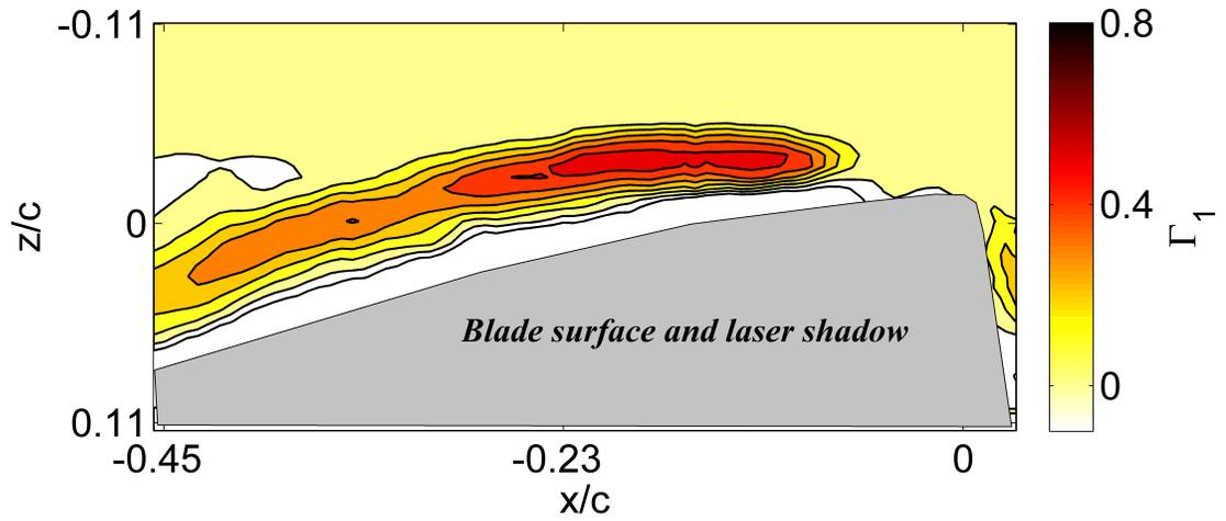
**Figure 24:** NAM plot at  $\psi = 235^\circ$ ,  $r/R = 0.6$ ,  $\mu = 0.35$
