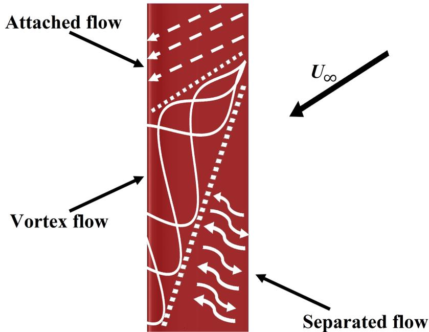
**Figure 101:** Proposed surface flow topology over a yawed wing in reverse flow
