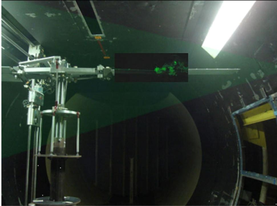
**Figure 66:** View of PIV imaging from camera
