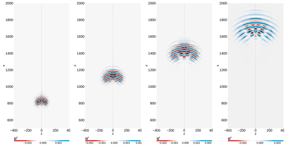
Figure 4.8: Nonlinear wave packet evolution at Mach 0.2, at y = 0.6\delta^*(x) . Contour levels at 90% (—) , 50% (---), 30% (...) and 10% (-.-) of the amplitude peaks in the packet.
