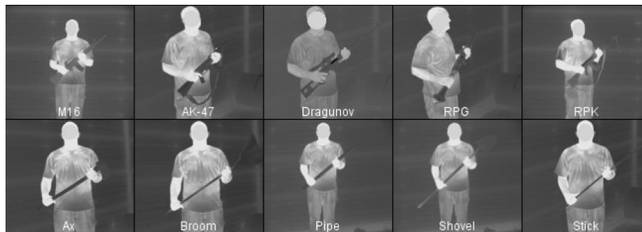
Figure 2-11 Thermal Images of Two-Hand Object Identification (Source: [P-37])
