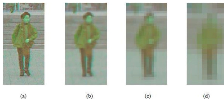
Figure 2-8 Test Image at Four Scales (a) Original Size (b) Factor-2 Reduction (c) Factor-4 Reduction (d) Factor-8 Reduction (Source: [P-19])
