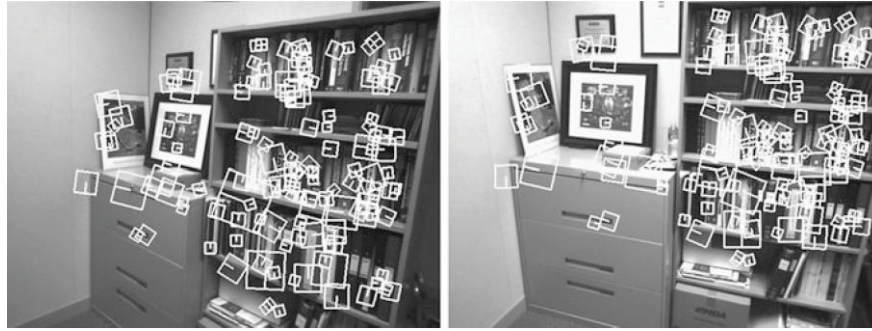
Figure 2-3 Example of Wide Baseline Matching Between Two Images With SIFT
