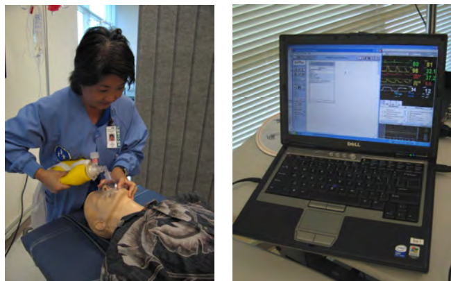
Fig. 1. SimMan™ manikin simulator and laptop computer, which controls the manikin via wireless technology
