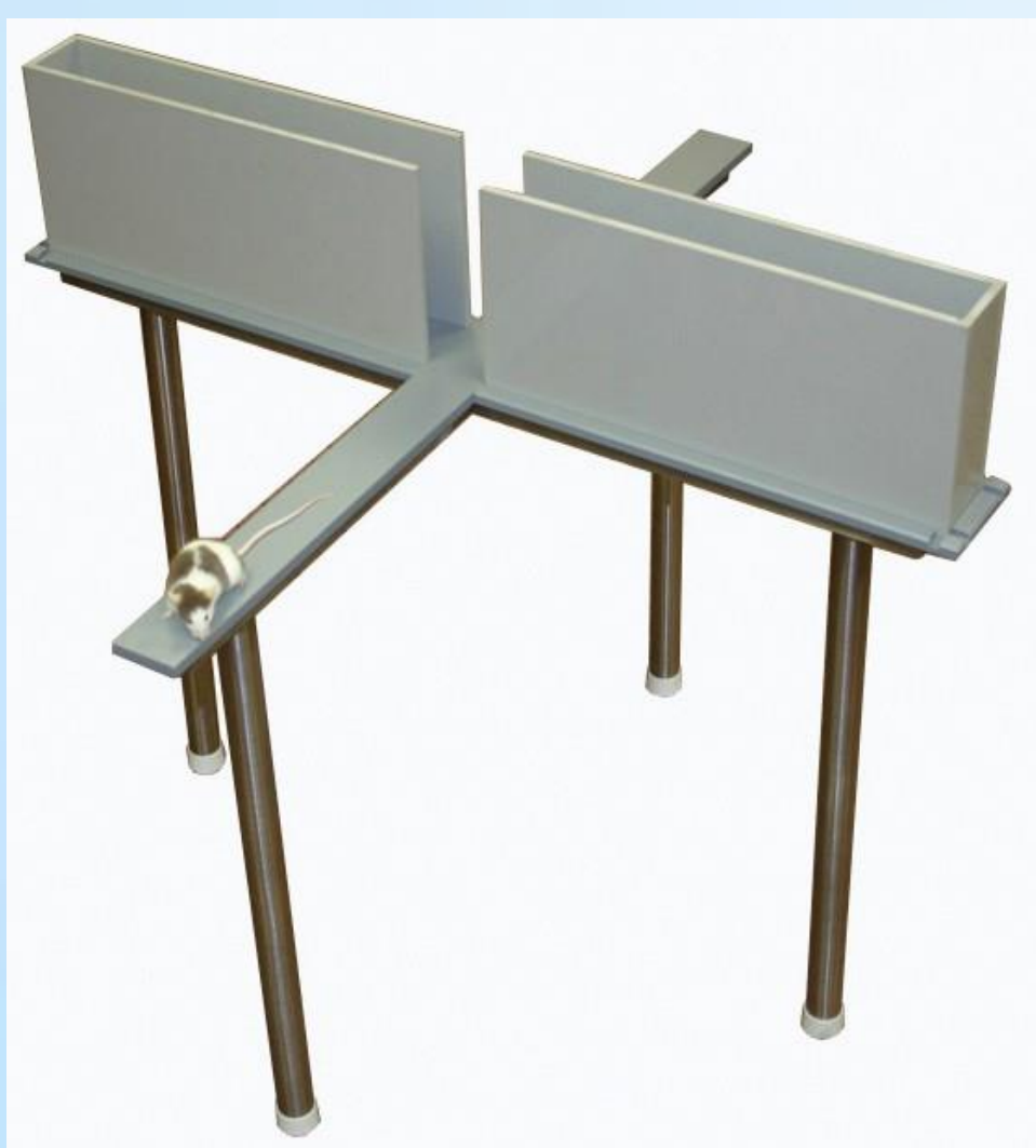
Figure 3. Elevated Plus Maze for anxiety measurements
