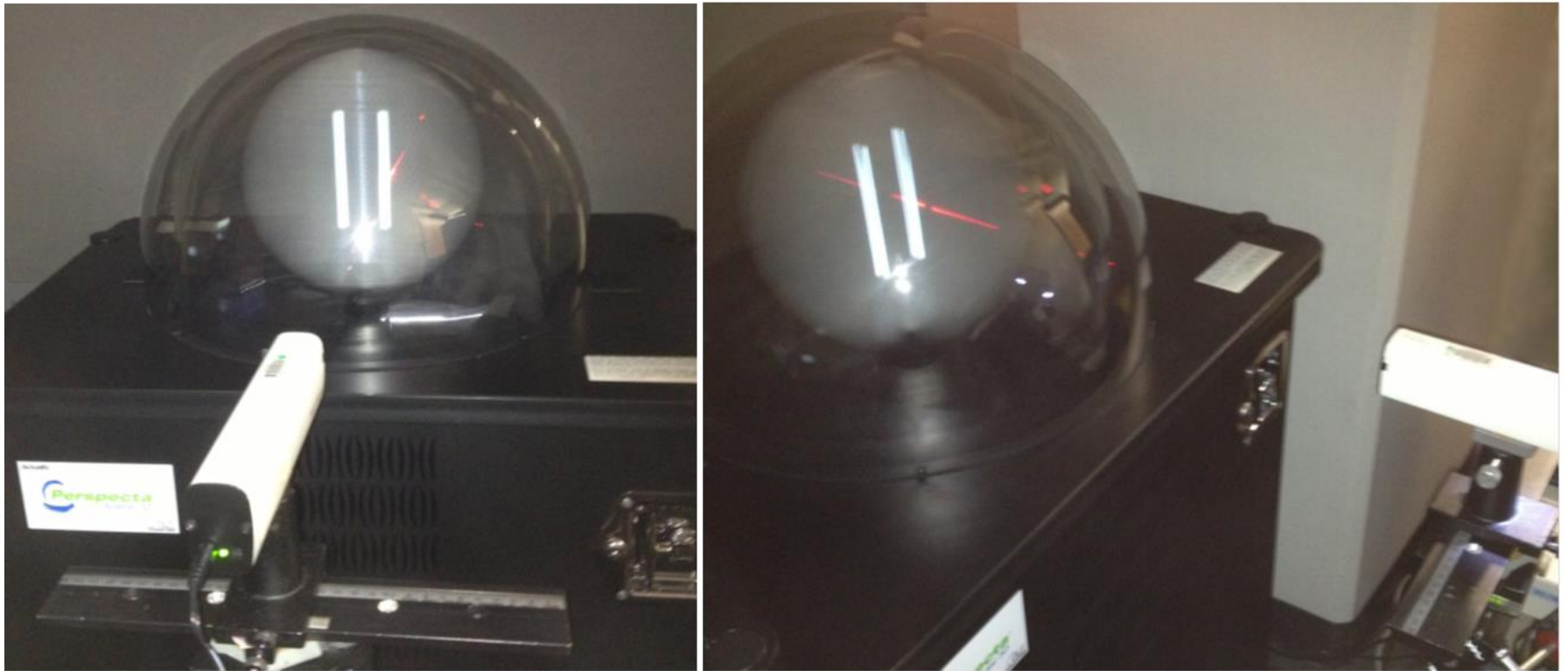
Figure 12. Remote Measurement of Rod Images on AIS Perspecta Using Orthogonal Laser Translation
