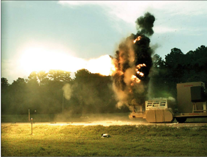
The rocket-propelled grenade defeat test of the FCS Active Protection System for Manned Ground Vehicles was the first time that any vertical launch APS defeated an incoming RPG while mounted on a moving vehicle.
