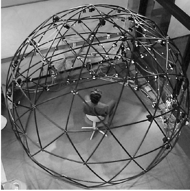
Figure 4: Geodesic dome with 64 flashes used to capture data base images.
