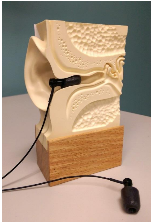
Figure 4. CEP (foam ear tips with communication cabling)
