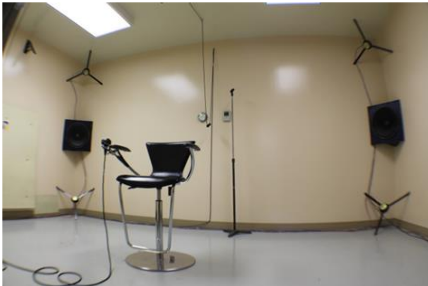
Figure 5. Facility used for measurement of passive continuous noise attenuation
