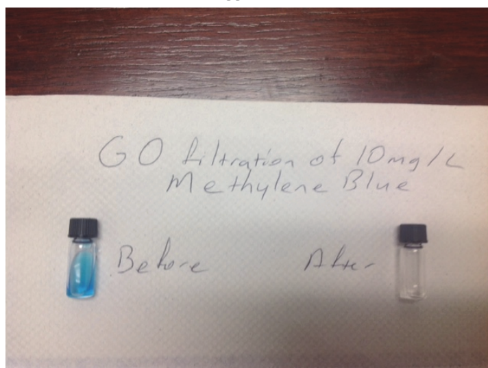
Figure 5. Use of Methylene Blue to assess effectiveness of Graphene Oxide Membranes (Study conducted by Petery and Griggs 2015).
