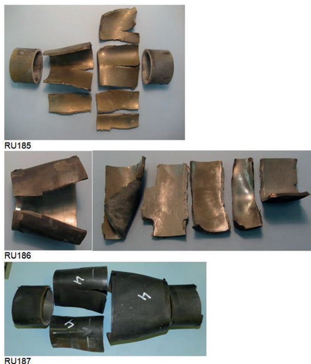
Figure 6. Steel cylinders after explosion-driven deformation with 5 mm Semtex layer in elongated configuration. From top to bottom are the experiments with RU185, RU186, and RU187, respectively.
