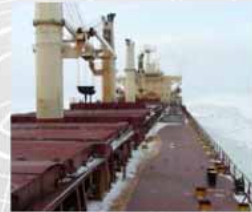
Nordic Barents Heavy ice-class bulk carrier
