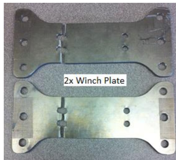
Figure 6: Winch Mounting Plate Post Tensile Test
