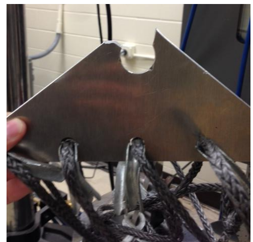
Figure 11: Block and Tackle Tensile Test Failure Location
