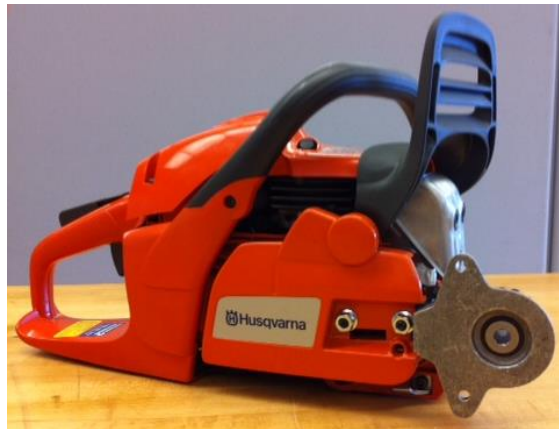
Figure 24: Husqvarna 460 Rancher Chainsaw With Winch Adaptor
