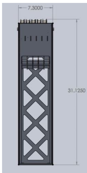
Figure 76: Pulley Lift Front Side Base Dimensions (in)
