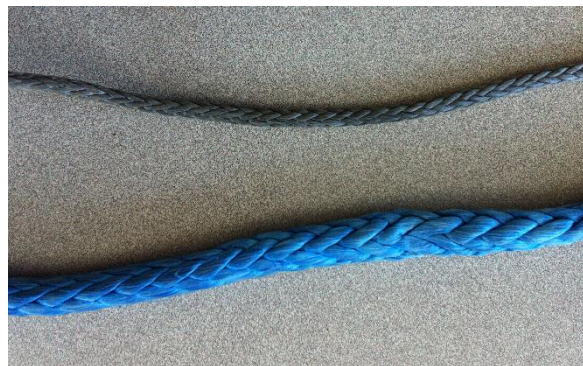
Figure 19: 0.5" and 0.25" Amsteel Blue Synthetic Rope
