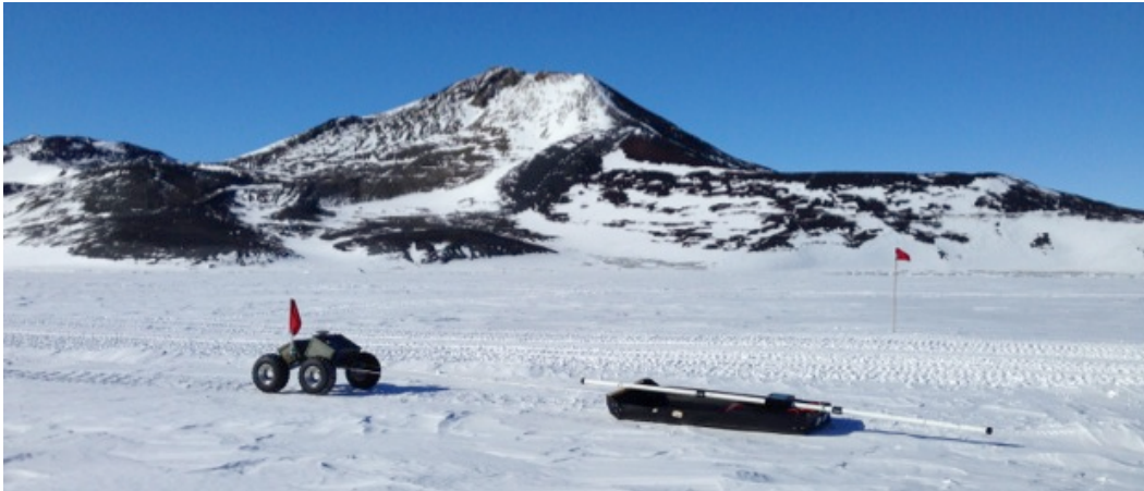
Figure 2. Yeti towing an EM31 electromagnetic ice-thickness meter along the Pegasus Cut-Off Road near McMurdo Station, Antarctic, on 11 November 2014.
