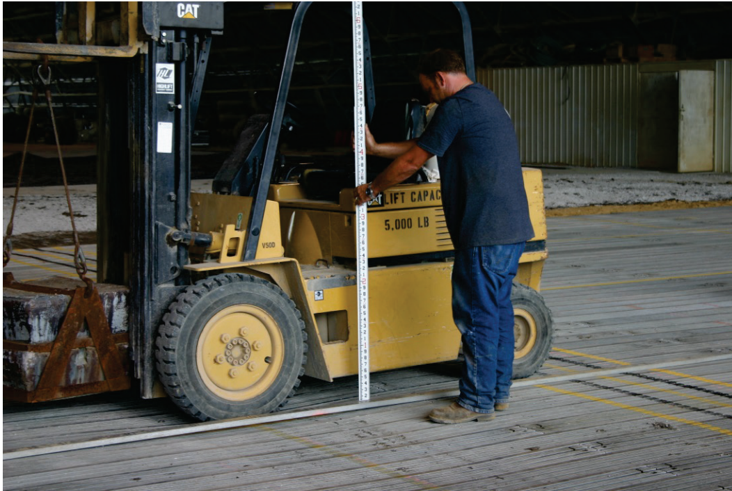
Figure 39. Loaded deflection procedure used to determine \delta_{s-2} .
