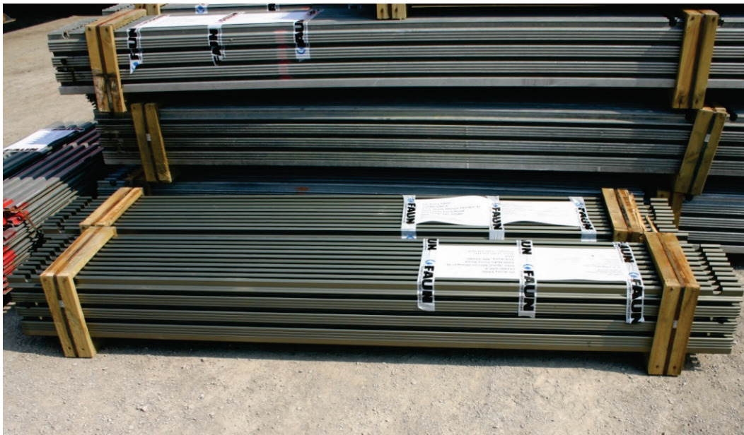
Figure 9. MLC-70 Trackway panels bundled for transport.
