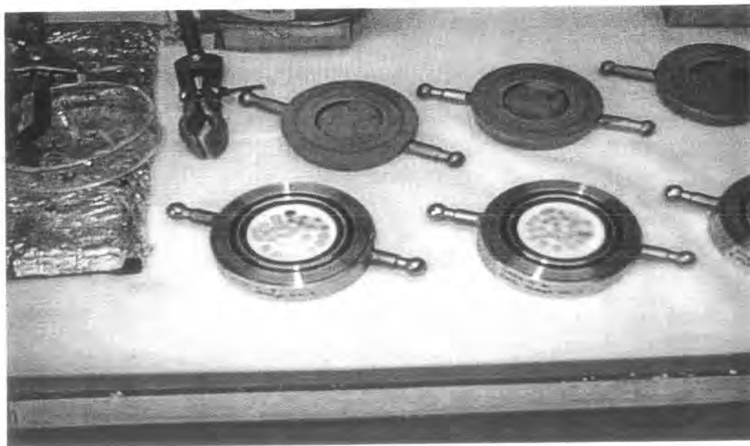
Figure 3. Photograph of GD Test Cells Showing the Transparent Areas
