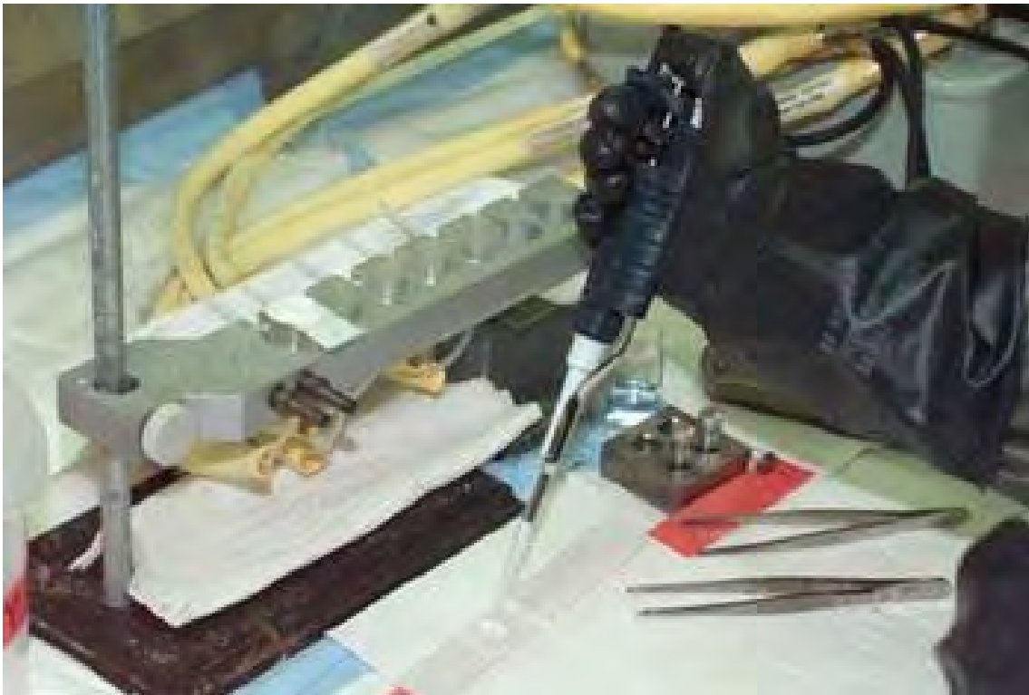
Figure 8. Penetration cell test. Cell holding assembly and dosing vapor cup with CWA.
