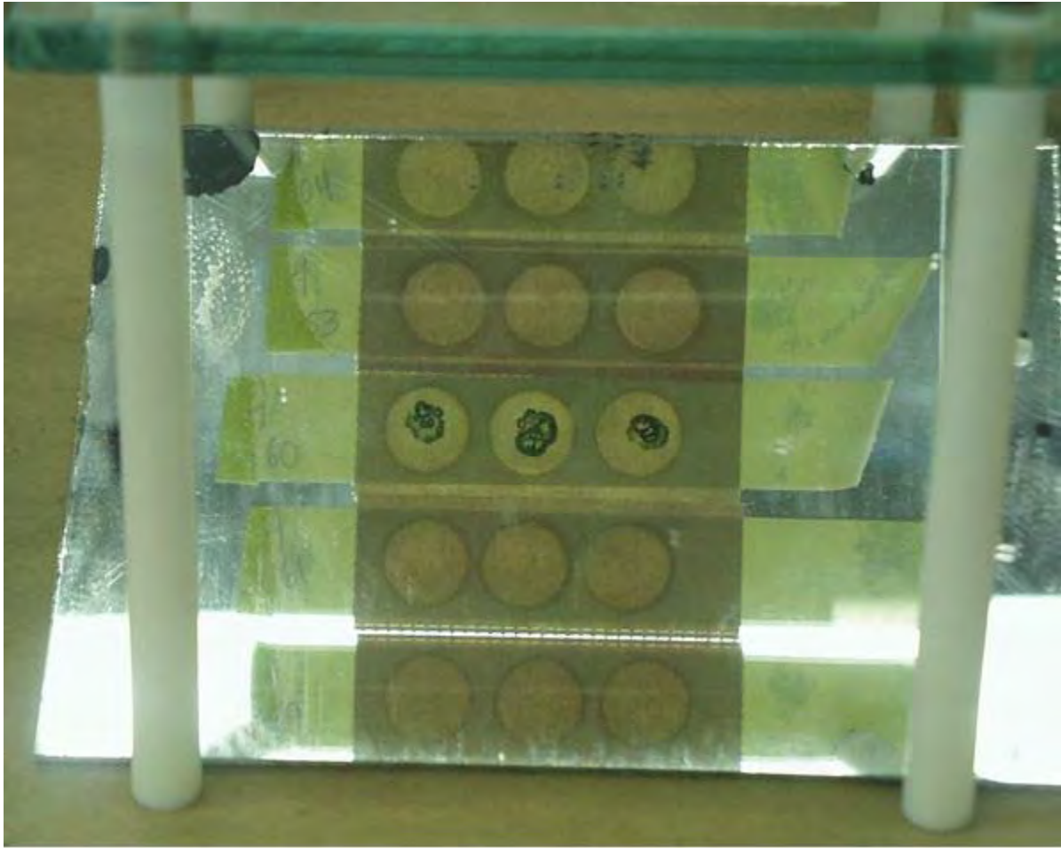
Figure 4. M8 test assembly. Breakthrough was observed from the bottom surface of the M8 paper using a mirror placed on an angle at the bottom of the test assembly.
