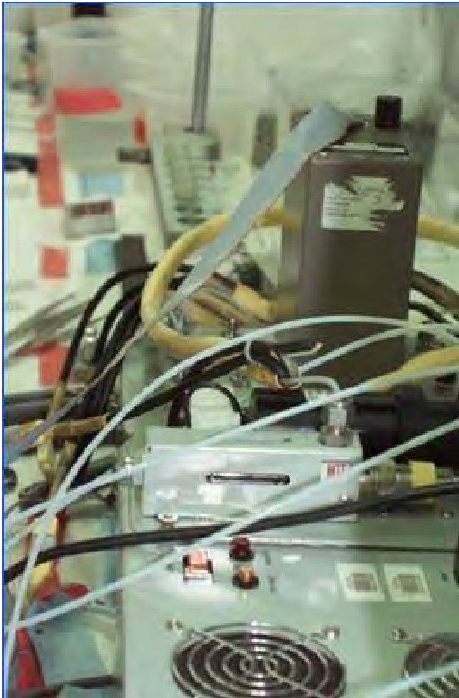
Figure 6. Micromer penetration cell test setup in hood.
