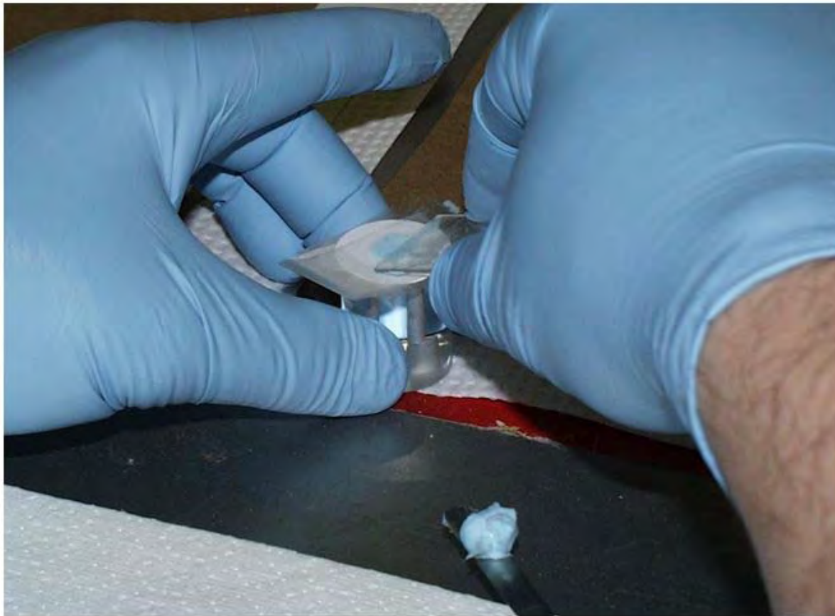
Figure 7. Removing excess aTSP from a glass penetration cell with cellulose acetate wafer and perforated tape strip.
