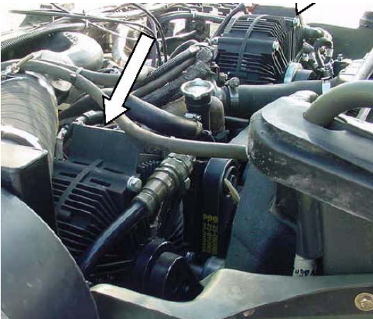
Dual belt driven HV generator
