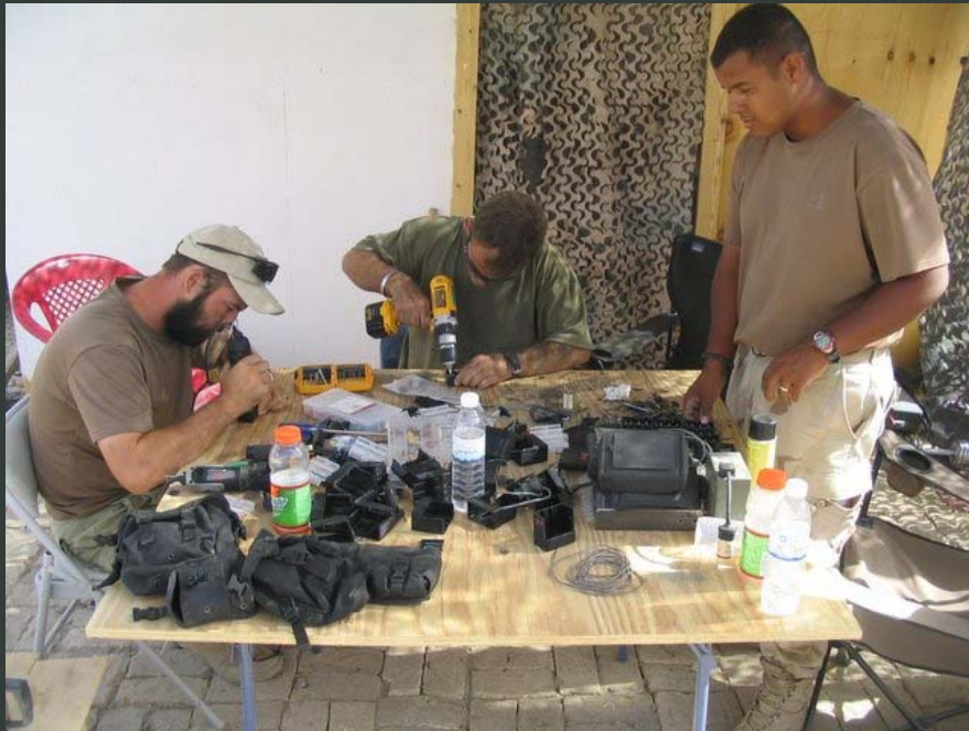
SF soldiers in theater ripping apart dozens of MBITR boxes to run them from BA-5590s
