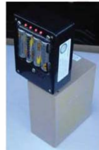
SCAVENGER – recharge AAs in 100 minutes scavenging unused energy from BA-5590 equivalent batteries.
