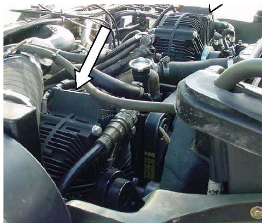
Dual belt driven HV generator
