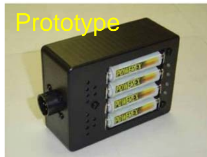
SCAVENGER – recharge AAs in 100 minutes scavenging unused energy from BA-5590 equivalent batteries.
