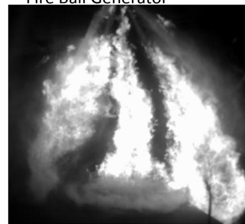
Fireball is based on a medium shaped charge penetration into fuel cell
