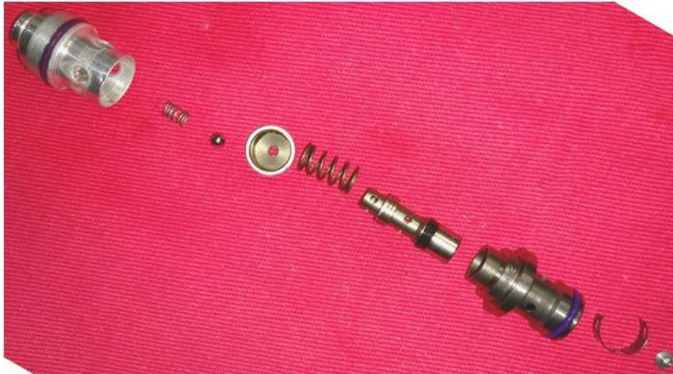
Figure 23. Disassembled Hydraulic Power Brake Pumping Element
