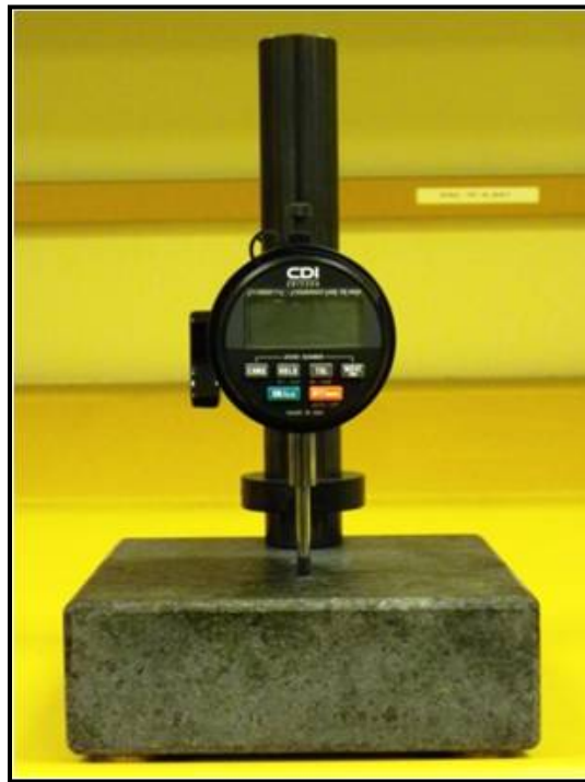
Figure A-1. CDI Micrometer to Measure O-ring Thickness
