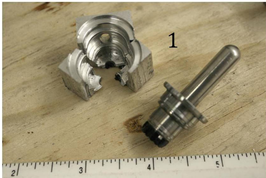
Figure 49. A hammer and chisel was then used to crack open the case and the valve and filter were then removed
