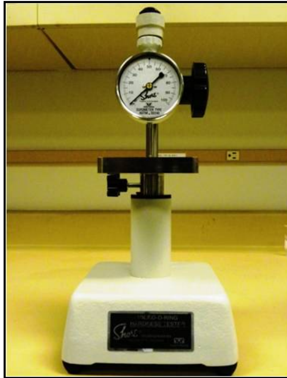
Figure A-2. Shore M Durometer to Measure O-ring Hardness
