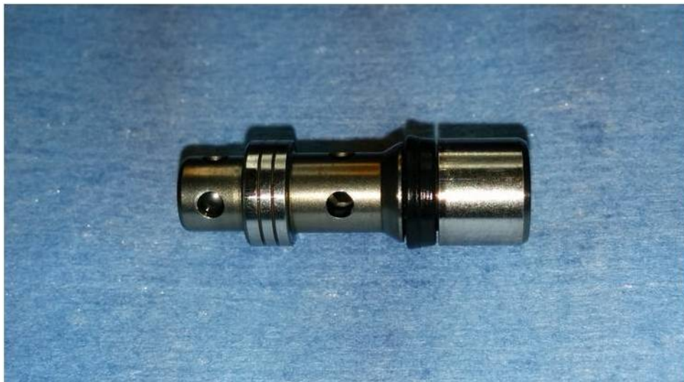
Figure 24. Hydraulic Power Brake Pumping Plunger Detail
