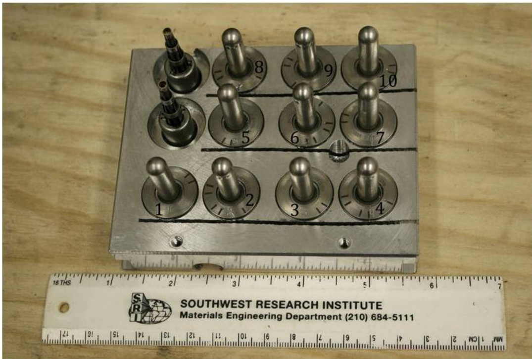
Figure 46. Parallel cuts were made along each row, with valves numbered as indicated
