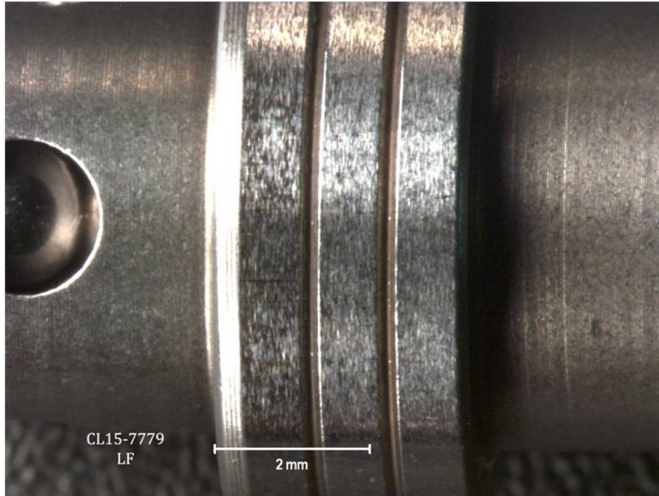
Figure 28. Detail of the Baseline LF Plunger Pumping Section Polishing and Wear
