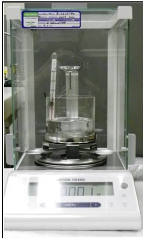
Figure A-3. Density Kit to Measure O-ring Volume
