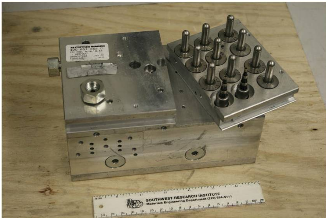
Figure 45. Valves sliced from the main block using a band saw
