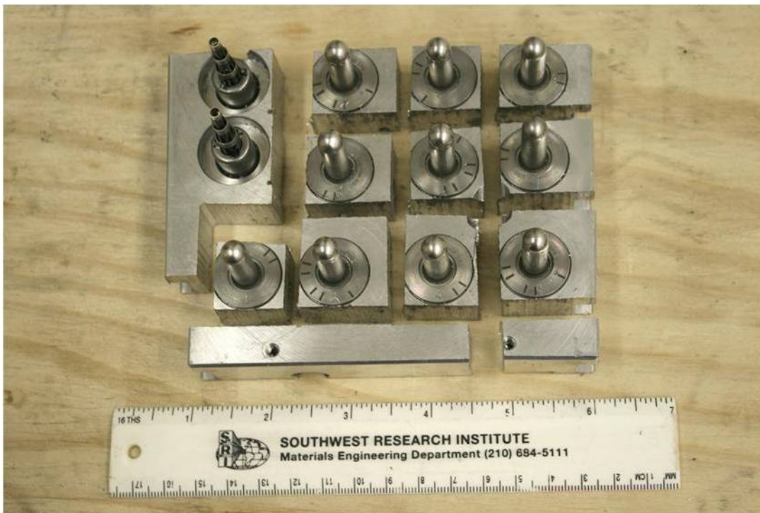
Figure 47. Cuts were then made perpendicular to the row cuts to isolate each valve and filter unit
