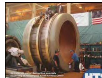
AMSC - 50,000 SHP (36.5MW) HTS AC Synchronous Motor
