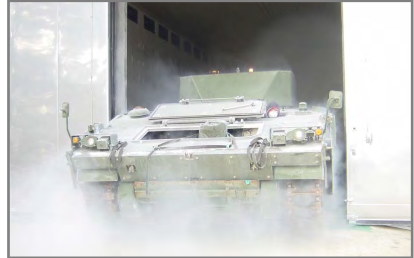
▲ An-Heung Low-Temperature Chamber
