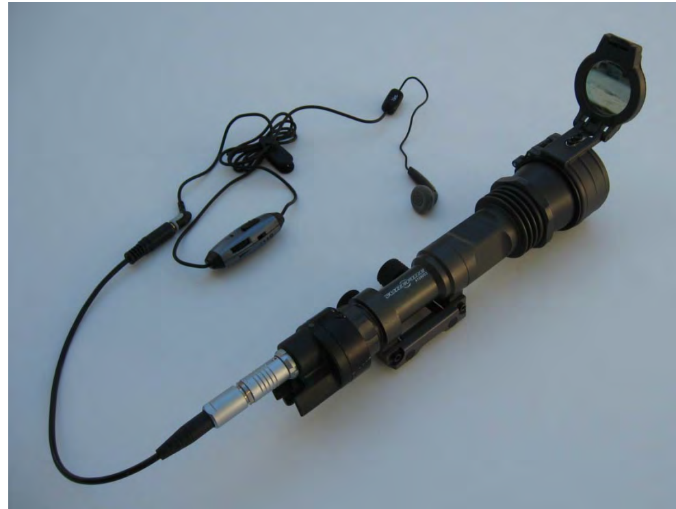
Operational LightSpeed SUREFIRE voice communication system
