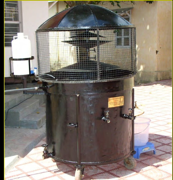
Iron Removal Unit
