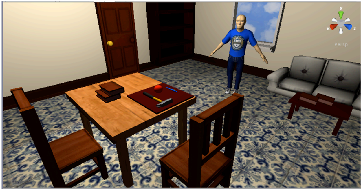
Figure 1 A virtual avatar will reach and grasp objects in virtual environment as shown here. The objects are designed such that grasping (ball, hammer) and pinching (pen) actions of the hand can be emulated in virtual environment. This environment was created in Unity3d.
