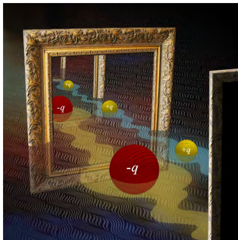
Figure 1: Charged particles in a liquid are enveloped by a cloud of opposite charge that deforms near boundaries, and creates a force away from the boundary. Electrostatically, boundaries act as mirrors, causing additional attractions or repulsions. Theory reveals how ions influence forces between boundaries in an intricate way, and vice versa, with important implications for biological systems (Artistic impression by D. Spjut).
