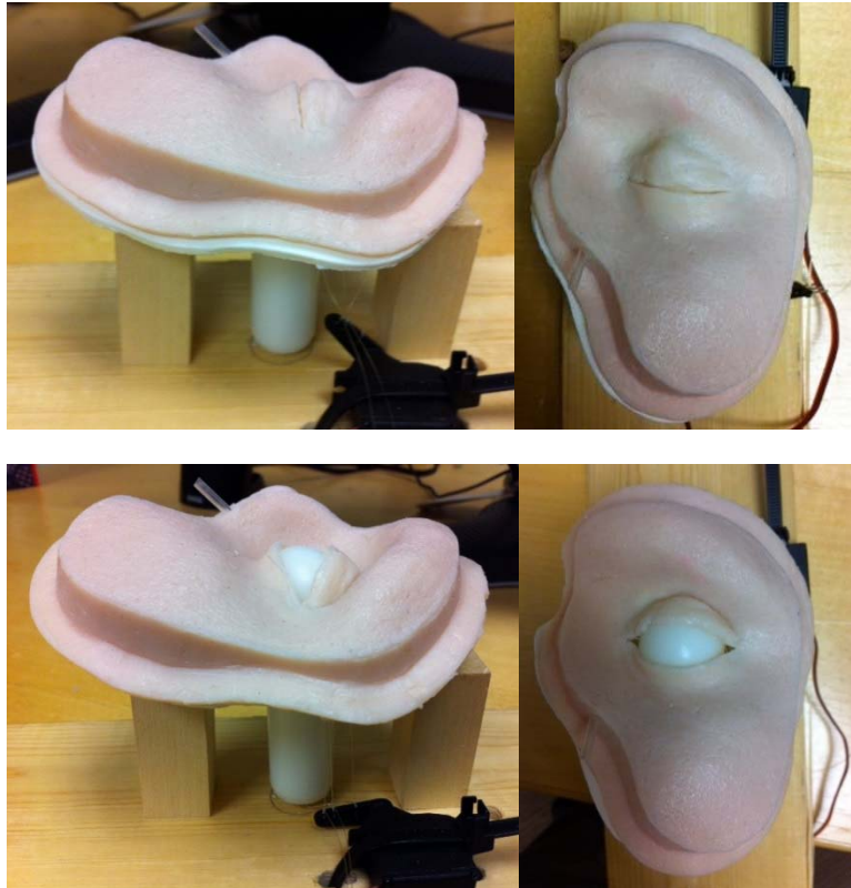
Figure 146: Servo control of module eyelid blinking
