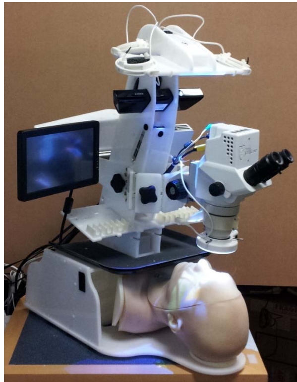
Figure 153: Standalone system with full suite of AR components installed: Kinect operating through mirror to enable hand tracking; projector displaying virtual buttons for non-contact interaction (illumination projected on table-top and face); AR microscope with position tracking to enable synchronized motion of microscope and imagery overlaid on direct view of facial anatomy.
