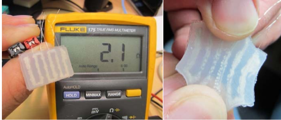
Figure 104: measuring resistance of serpentine conductive ink trace embedded within silicone. Silicone stretches as normal skin, but conductivity is lost as ink trace is fractured.
