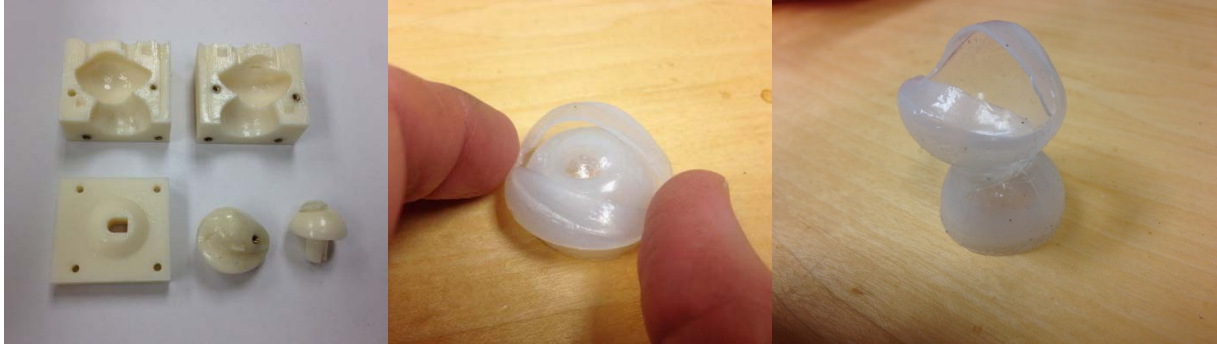
Figure 74: Year 4 eye globe mold, disassembled (left); Year 4 eye-globe and conjunctiva, detail (middle); eye globe and conjunctiva (right)
