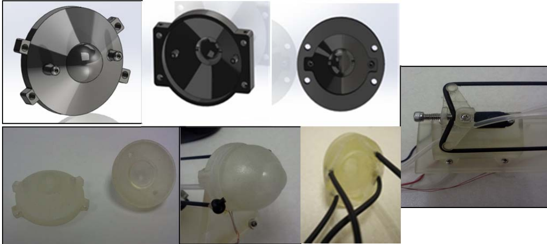
Figure 42: base plate modifications, rapid prototyped test versions of plate and globe showing plate and globe segment separately and assembled. Features include bosses for neoprene cords to replace latex rubber bands. Modified elastic transmission components: o-ring cord threaded through servo arm, initial baseplate attachment.
