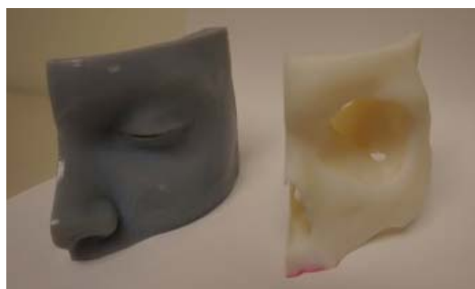
Figure 39: Early concept for division of head elements using Solidworks CAD tools; rapid prototyped rubber and hard plastic sections created from CAD models.
