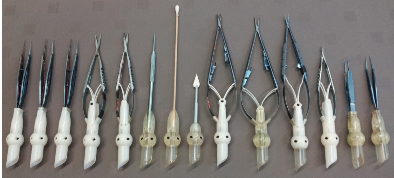
Figure 33: Instrument holder designs for new devices (cotton swab, punctal dilator), earlier devices for globe surgery (straight and bent tying forceps)
