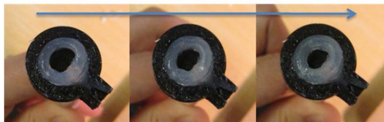
Figure 56: Sequence of inflation of toroidal "iris" to cause contraction of pupil.
