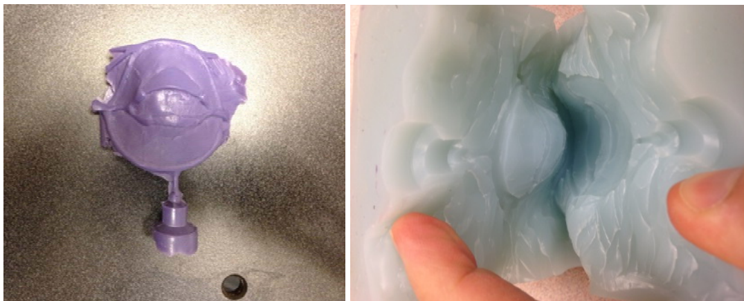
Figure 68: Mold insert for revised canalicular routing in tarsal plate, prior to removal of flashing; mold for replication of revised design.
