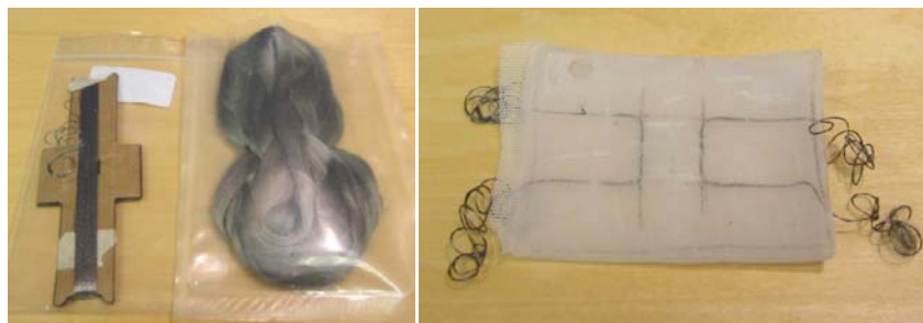
Figure 105: Conductive thread and unweaved fiber; fibers embedded in silicone for testing.
