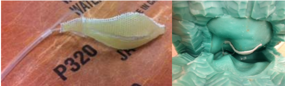
Figure 60:(Left) eye tarsal plate, with attached lacrimal, nasolacrimal duct tubing, reinforcing mesh (as per previous versions of the portal) (Right) Mold for eyelid portal, with tarsal plate, ducts in place for over-molding with softer durometer silicone for eyelid/skin structures. Sprues from tarsal plate molding process hold the plate and duct structure in place for overmolding process.
