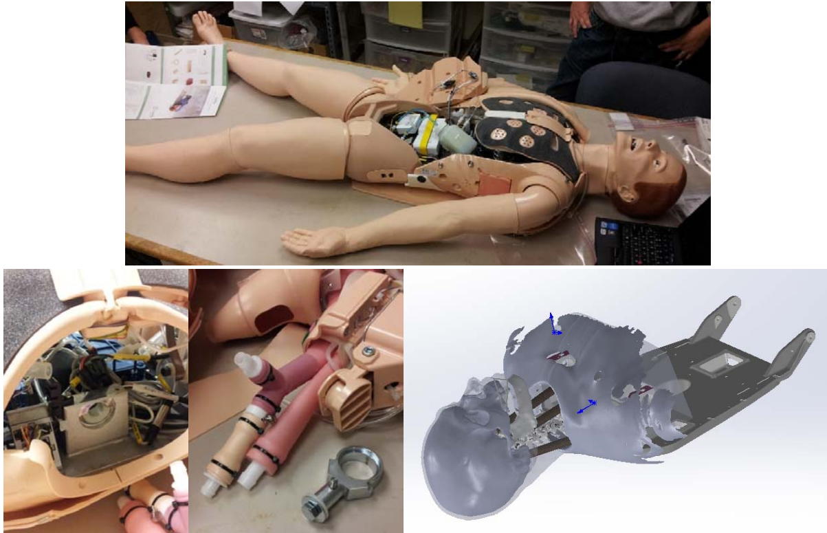
Figure 149: Disassembly and examination of Laerdal SimMan Essential mannequin in support of designing interface components to mate the new head/neck to the commercial body. Aligned CAD models in use for design of attachments between new head/neck and stock mannequin.
