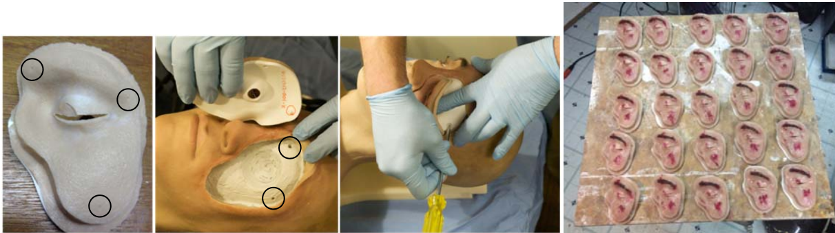
Figure 5: (left to right) Y1 module design with dimples for position calibration – instruments contact at each location to confirm position and orientation; attachment/alignment features to maintain stability of module during scenario; installation of module; 25 modules prepared for USUHS user testing.
