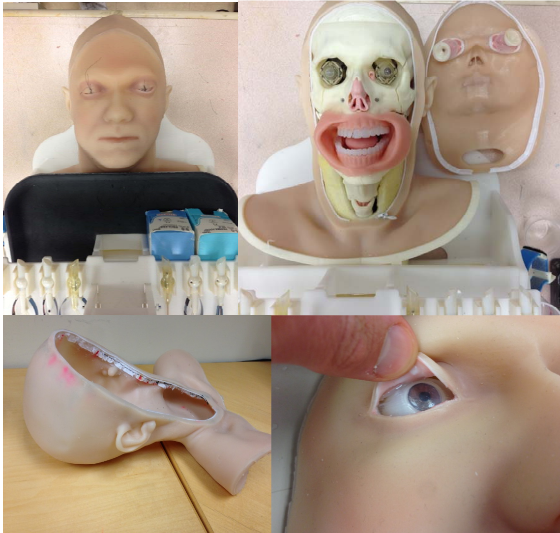
Figure 80: (clockwise) new face and cowl installed; new face and cowl partially disassembled; eye/eyelid detail; cowl disassembled.
