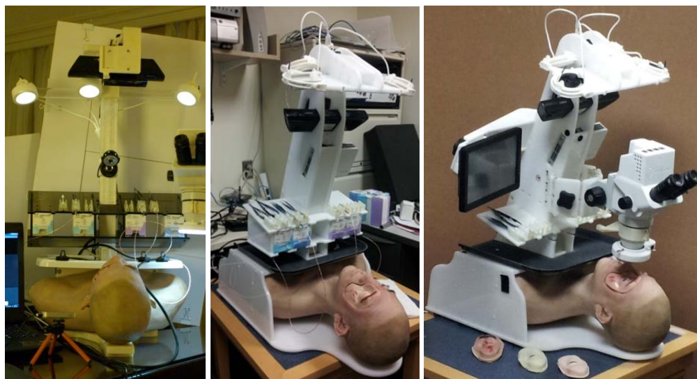
Figure 26: (left) Early Year 2 stand, ca. 1/2013. (middle) Year 2 stand, ca. 5/2013 for 2 nd USUHS Ocular Trauma Course. (right) Year 3 stand ca. 6/2014, with modified instrument rack, integrated touch-screen display and augmented reality microscope. The 6/2014 version allows for drop-in replacement of the head form with the more advanced version described below.
