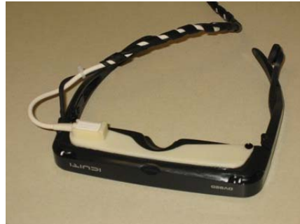
Figure 84: commercial VR glasses with mounting frame for magnetic position tracker and model 800 sensor from proof-of-principle simulator (larger sensor appropriate for this use vs. attachment to surgical instruments).
