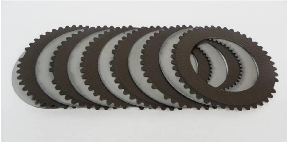
Figure 4. TEST Transmission C1 Clutch Assembly
