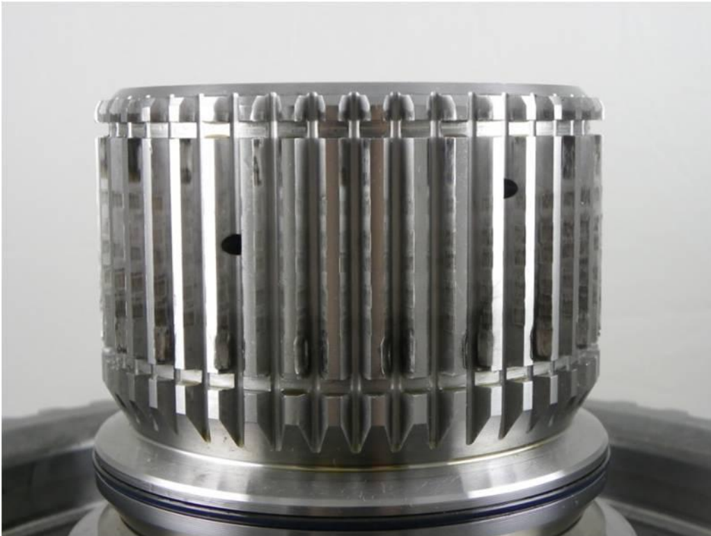
Figure 29. TEST Transmission Balance Shaft Spine Wear
