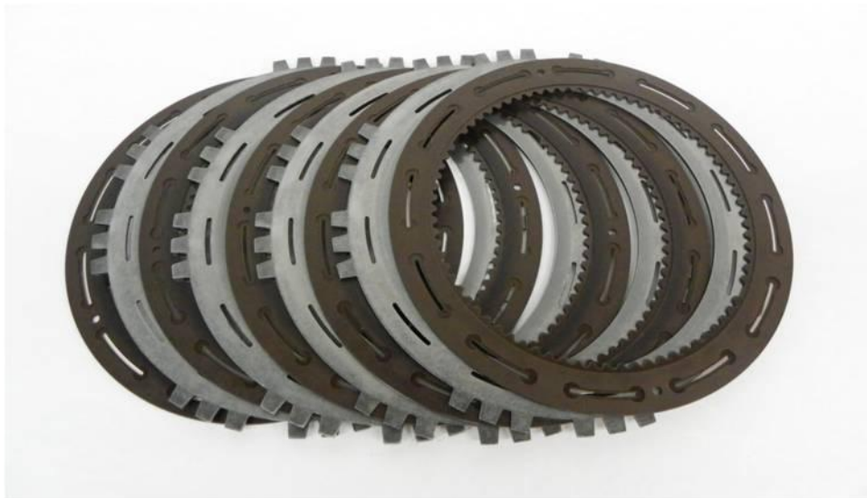
Figure 14. TEST Transmission C4 Clutch Assembly
