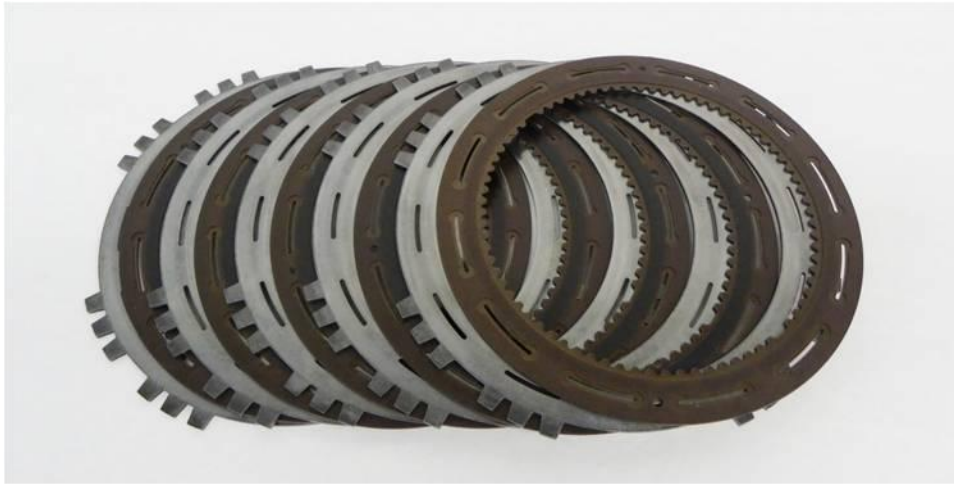
Figure 11. CONTROL Transmission C3 Clutch Assembly
