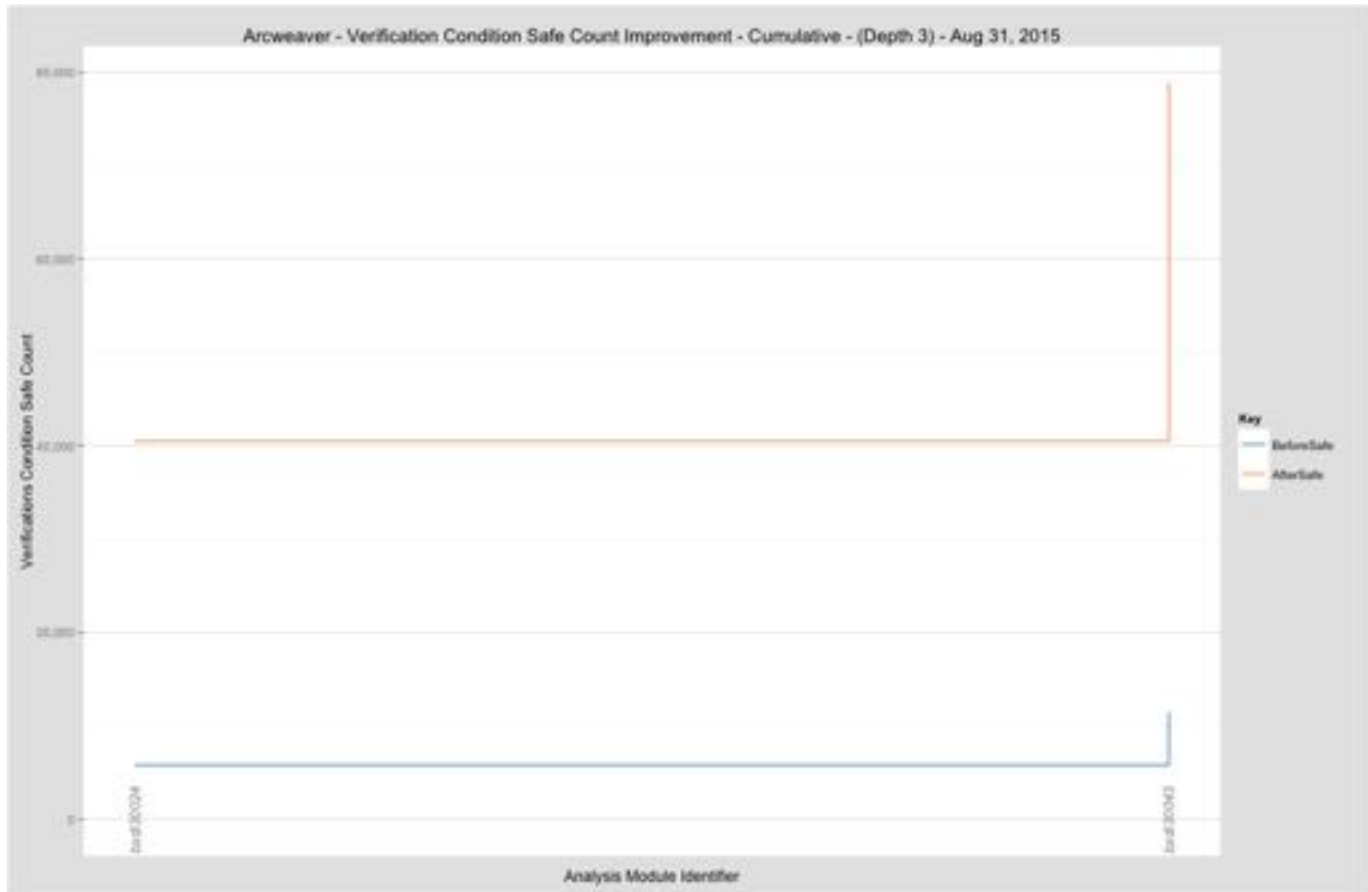
Figure 124: Arcweaver auto-solver results presented as before-and-after safe verification condition count cumulative improvements by module with three levels of inlining. The module arrangement is by identifier. The blue line represents the cumulative count of safe verification conditions before game play. The orange line represents the cumulative count of safe verification conditions after game play. The overall result is roughly 11% improvement in total verification closure. Data and analysis through 31 August 2015.
