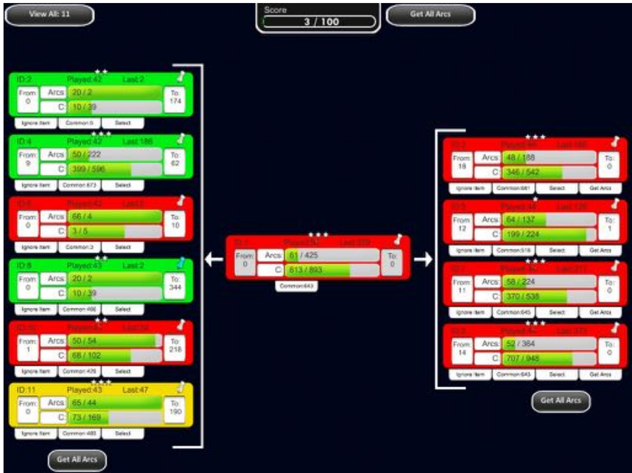
Figure 45: VIPER game play. This workspace shows a single instance in the middle and the related instances up and down the call graph. Color coding shows red for instances which link to or produce no arcs beyond the ones contained initially. Yellow shows arcs from the server points-to graph, and green represents instances which have produced additional arcs after importing arcs from server's global points-to graph.
