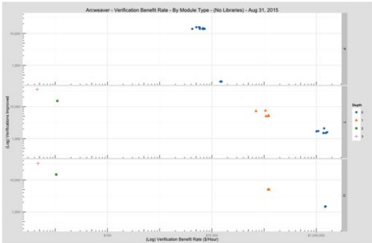
Figure 136: Arcweaver auto-solver verification benefit rates represented as the log of verification benefit dollars per hour versus the log of verification conditions improved, by program type panel. Samples are distinguished by constraint generator depth of inlining 0-3. Program types are U for utility, T for test, and P for program according to the BIND manual. Library module types are not included. The benefit dollars per hour are computed by our verification condition to SLOC scale model described in the text. Data and analysis through 31 August 2015.
