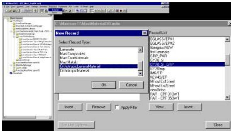
**Figure 7.2: Inserting an *OrthotropicLaminaMaterial* into the MASTSAS Database**
