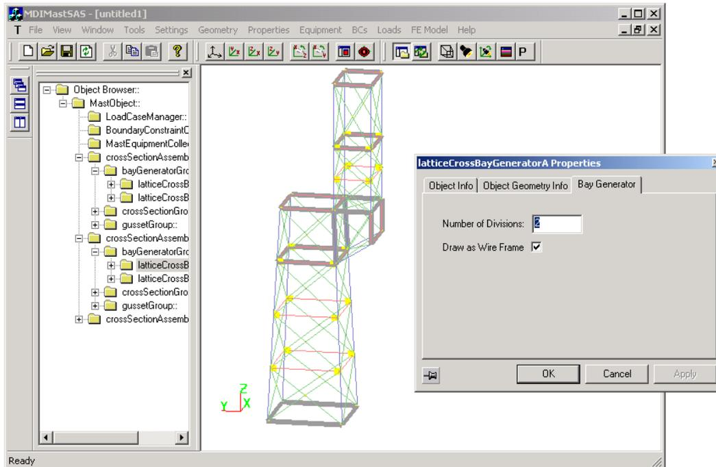
**Figure 2.26: Subdivision of lower bay of auxiliary mast**
