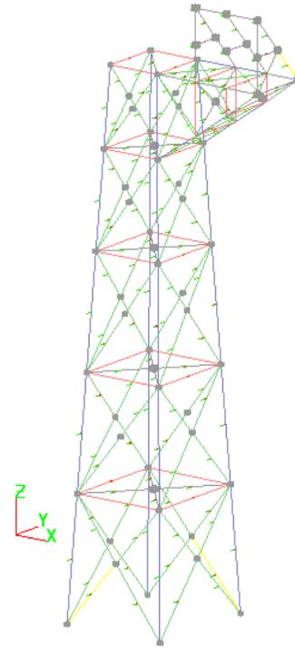
**Figure 4.12: Blast overpressure applied to the Dicethrow Mast**
