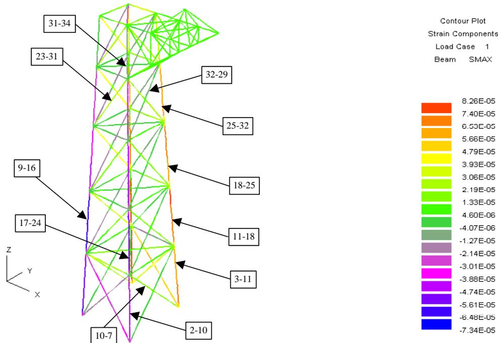
**Figure 4.11: Maximum strain contours for Event Dicethrow Mast**
