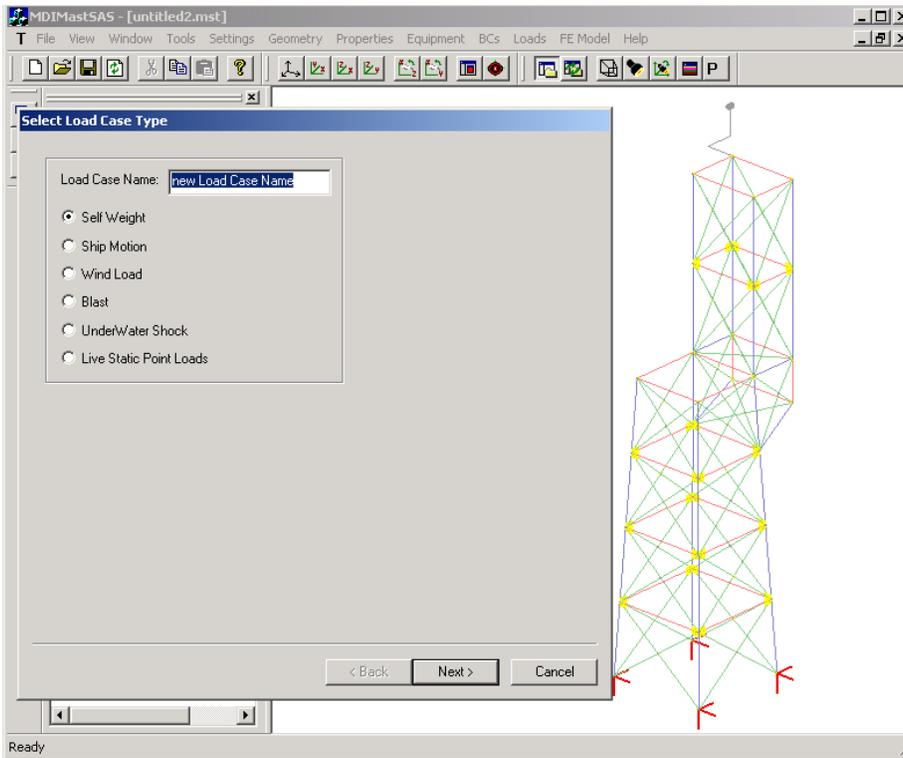
**Figure 2.37: Load case definition (simple lattice mast)**
