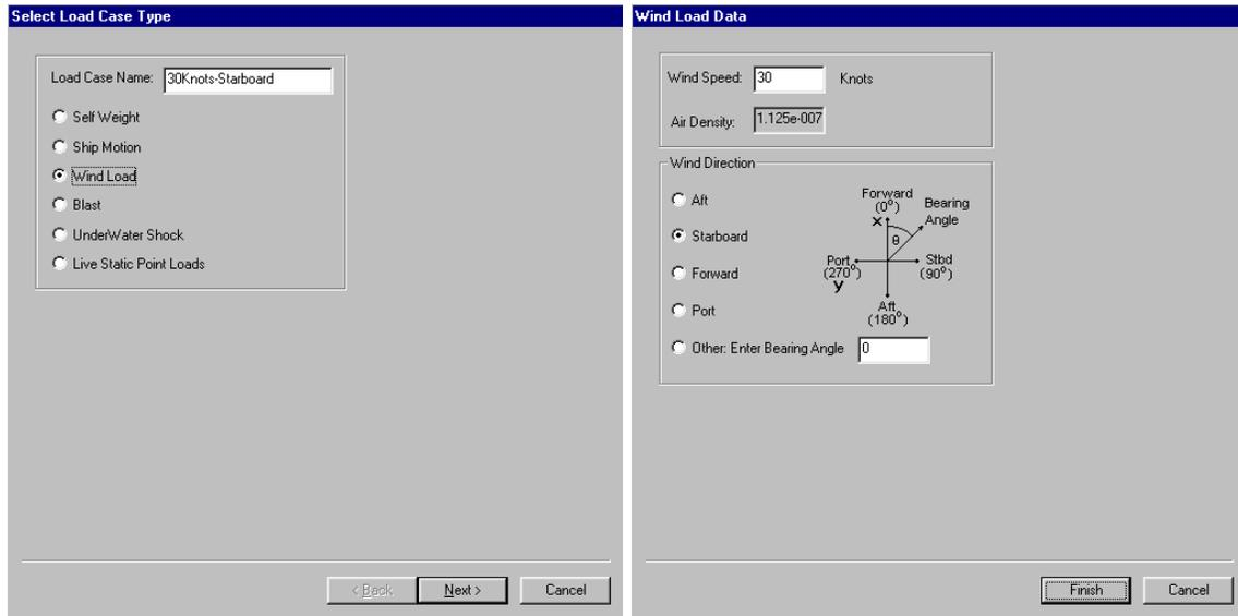
**Figure 4.15: Application of 30-knot starboard wind load**
