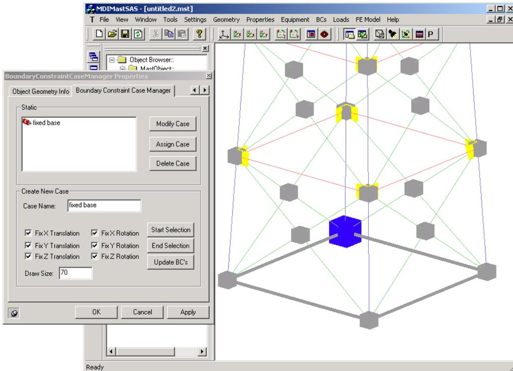
**Figure 2.33: Nodal identification for application of boundary conditions**
