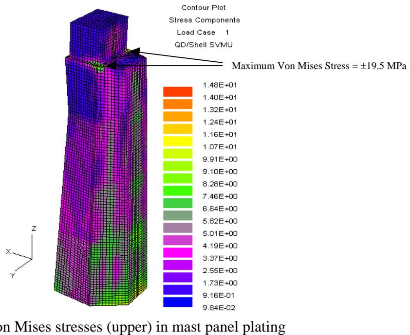
**Figure 6.7: Stress contours from 120-knot aft wind applied to the Dutch Mast**
