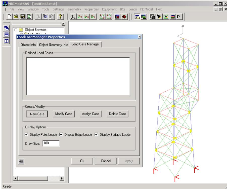
**Figure 2.36: Specification of new load case**
