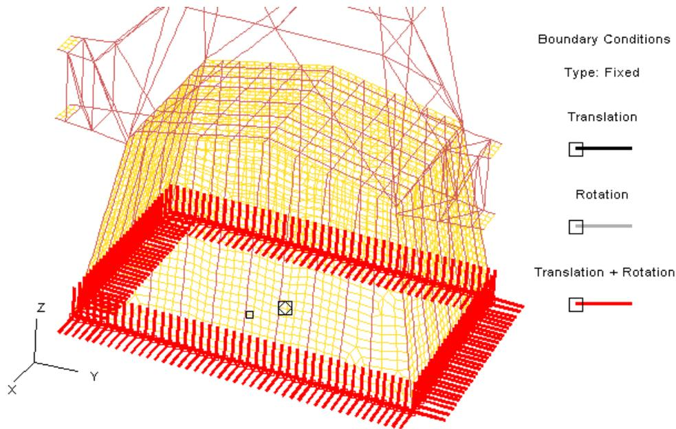
**Figure 5.11: Boundary conditions applied to CPF model**
