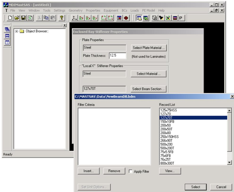
Figure 3.8: Specification of plate and stiffener properties
