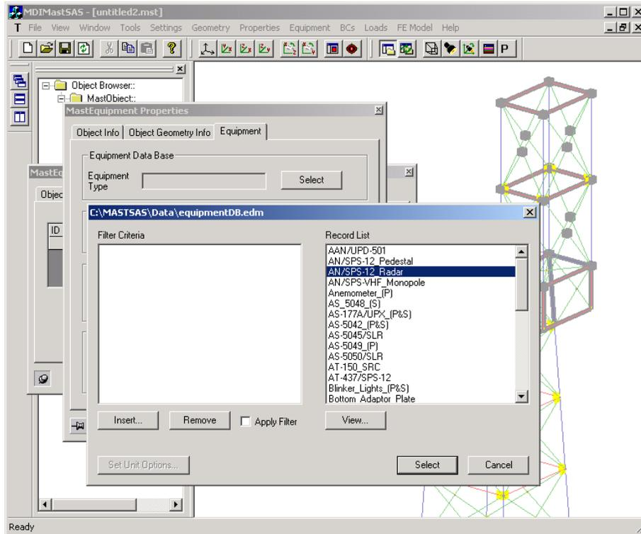
**Figure 2.30: Selection of mast equipment from database**
