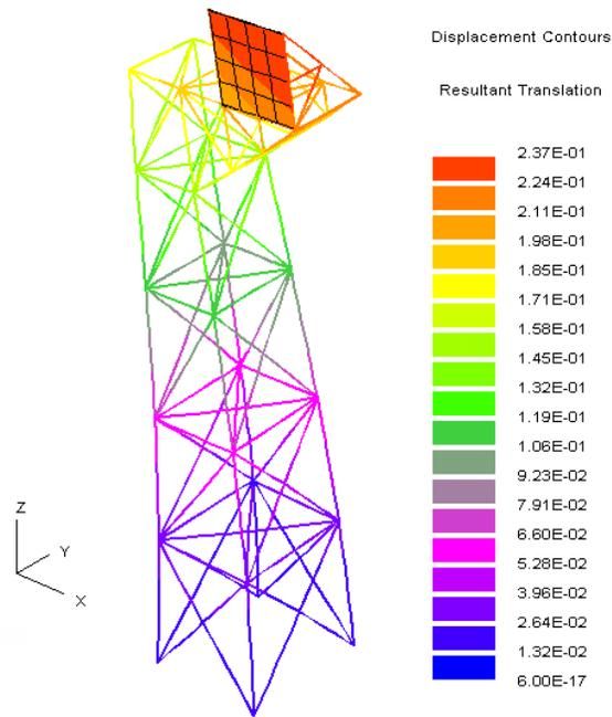
**Figure 4.21: Displacement contours under sea state 5 ship motions**
