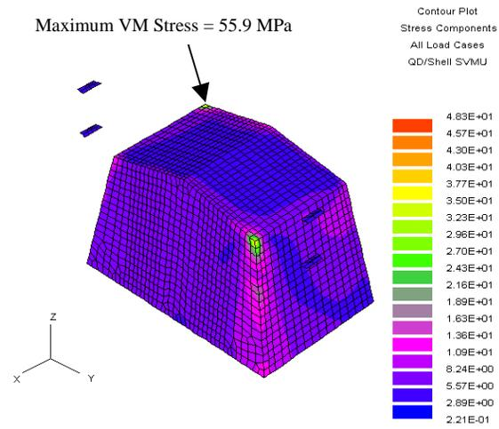
(c) von Mises stresses (upper) in ECM compartment plating
