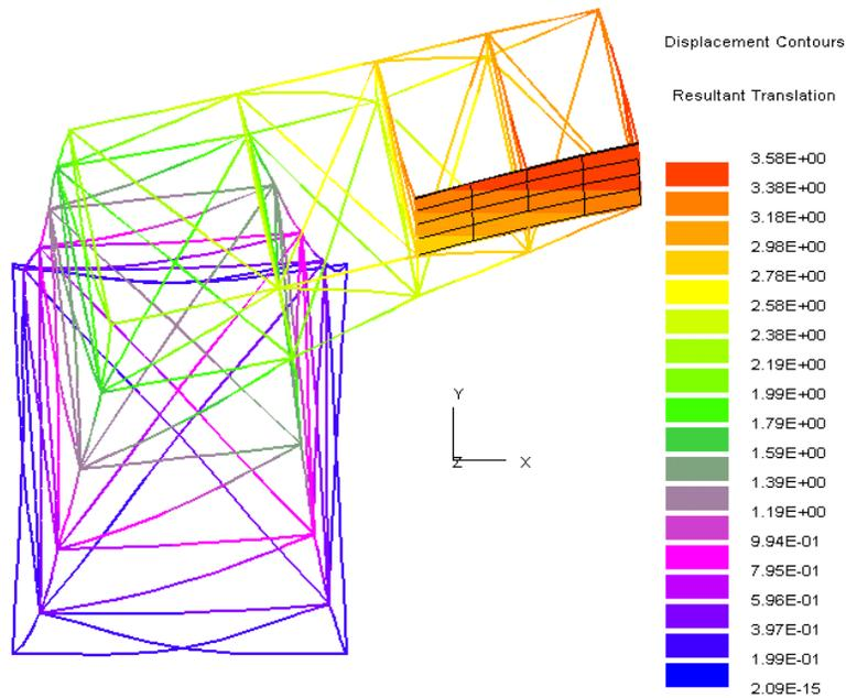
**Figure 4.18: Displacement contours showing twisting of Dicethrow mast**
