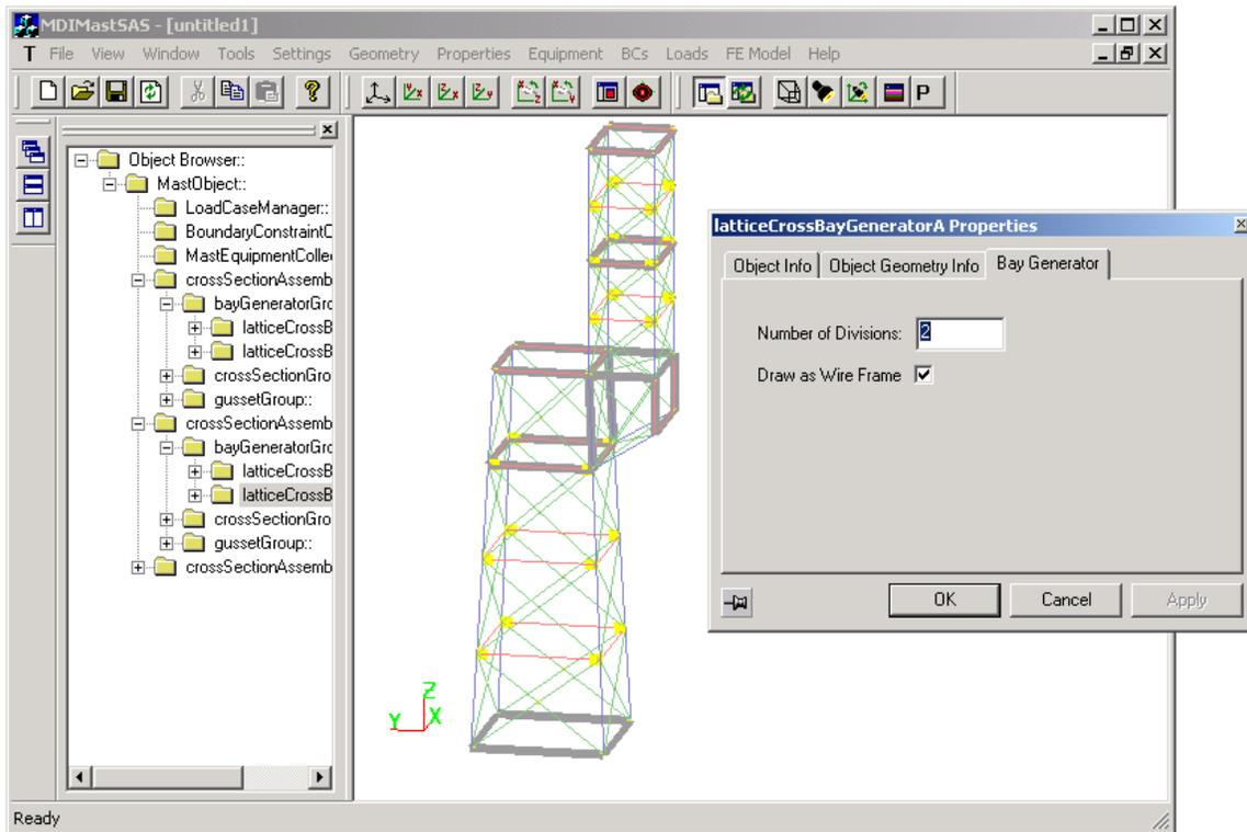
**Figure 2.27: Subdivision of upper bay of auxiliary mast**
