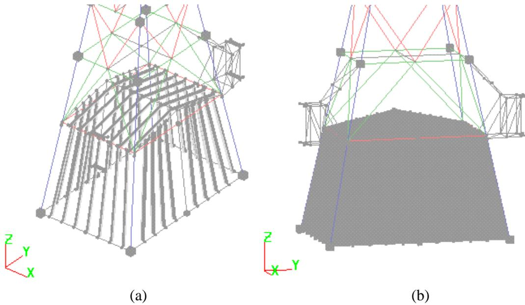
**Figure 5.9: Stiffened panel configuration for ECM compartment on CPF Mast**
