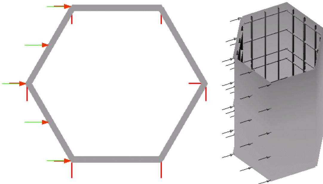
**Figure 3.21: Resulting wind loading on mast structure**
