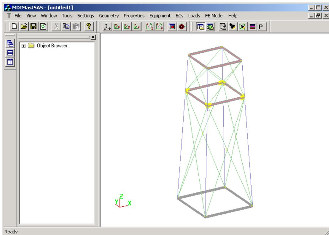
**Figure 2.8: Resulting main mast section (simple lattice mast)**
