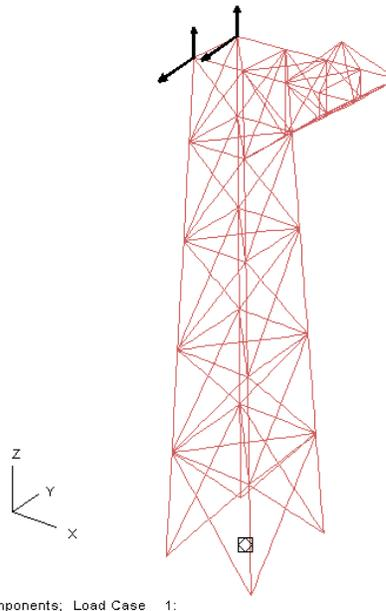
**Figure 4.10: Static loads applied to Event Dicethrow Mast**
