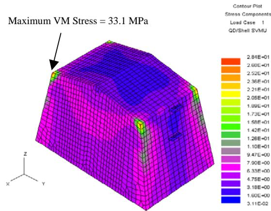
**Figure 5.14: Stress contours resulting from 120-knot starboard wind applied to the CPF Mast(cont.)**
