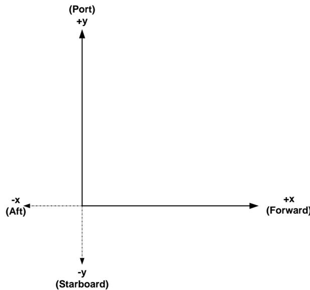
**Figure 4.3: Cartesian coordinate system versus ship axes system**
