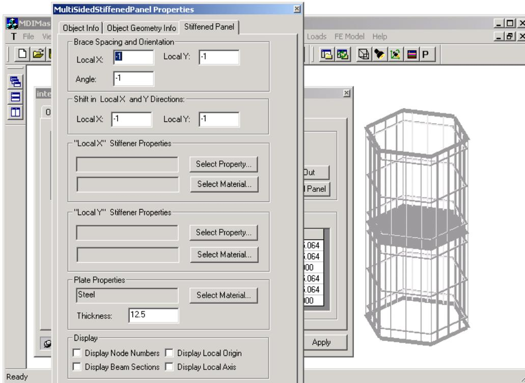
**Figure 3.12: Definition of interior stiffened panel properties**
