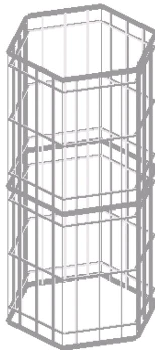
**Figure 3.10: Main mast section of simple enclosed mast model**
