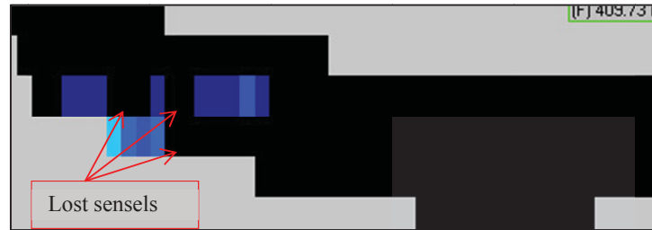
Figure 15: Oblique 55° non-penetrating ballistic test showing lost sensors.
