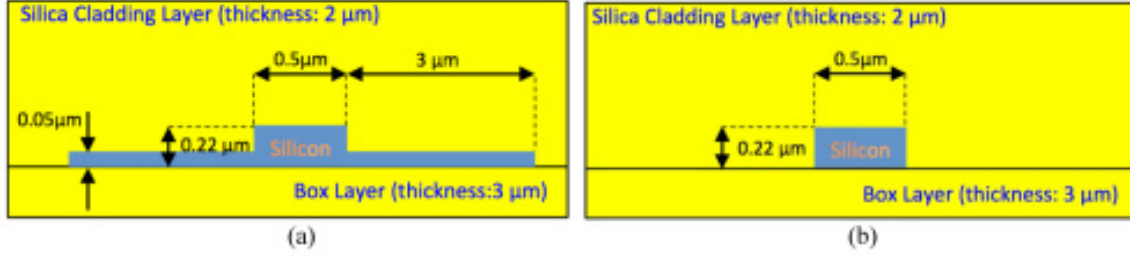
Fig. 1 Cross-sections of two kinds of waveguides used to build MZIs: (a) the rib waveguide, (b) the strip waveguide.
