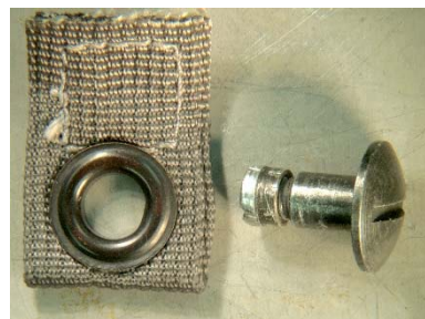
Figure 9. An ACH screw/nut set that pulled through the grommet.
