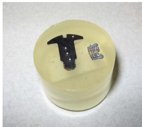
Figure 3. Example of cross-sectioned screw (ACH in this example) and nut mounted in plastic and polished. The marks on the surface of the screw are Rockwell hardness indentations.
