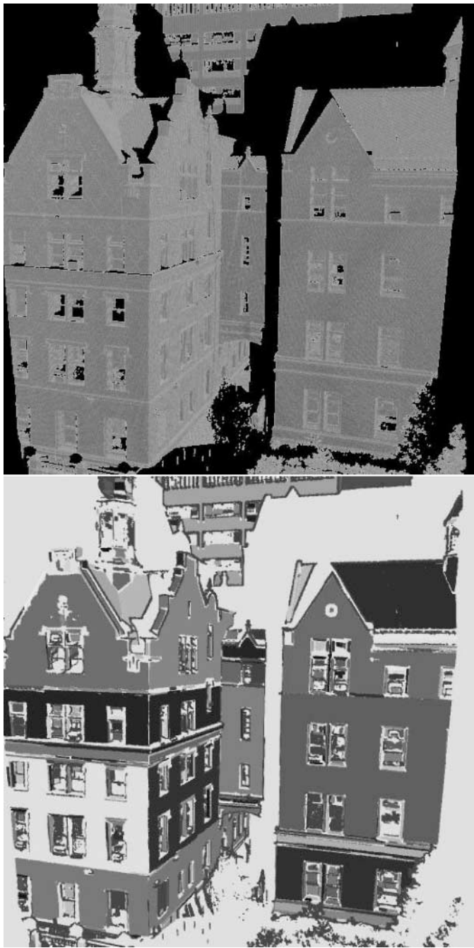
FIG. 7. Teachers College. Range (top) and segmented (bottom) image of the scene. Each segmented surface is displayed with a different color. The points which failed the initial Point Classification step are displayed in red.
