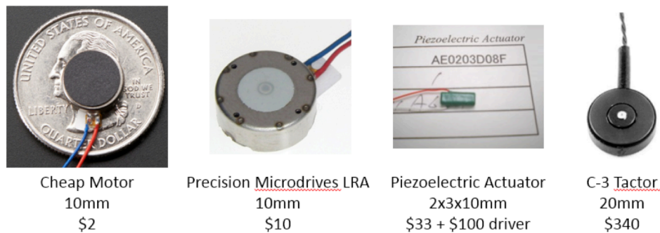
Figure 1: Four example haptic actuators we have purchased and examined in our lab.
