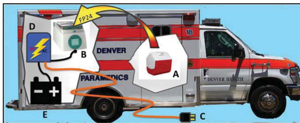
FIG. 3. Field plasma system schematic. FP24 is stored frozen at less than -18^{\circ}\text{C} in a high-performance cooler (A) passively chilled with a phase change material. This cooler is unpacked at the time of randomization and, if it contains FP24 (instead of a dummy payload for the control arm), these units are transferred to the Plasmatherm dry warm water bath system (B) where they are thawed in approximately 3 min. The Plasmatherm is powered by a self-contained electrical system that is charged by connection to conventional 110 VAC mains power via a shore power coupling (C) when the ambulance is parked. A power inverter/battery charger (D) both charges a lithium-ion storage battery (E), which supplies power to the system while the ambulance is in the field, and converts the battery's DC power output to AC to run the Plasmatherm.
