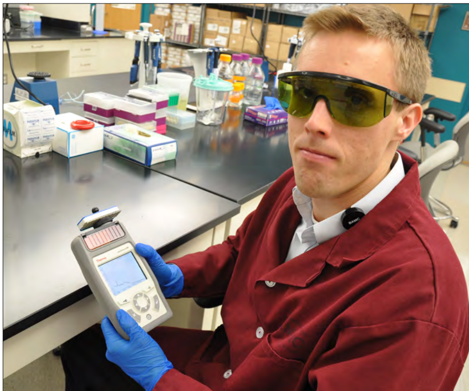
NAMRU-SA Bioengineer and Postdoctoral Fellow, Christian N. Kotanen, Ph.D., is holding a battery powered, hand-held Raman spectrometer that can display biomolecular "fingerprints" of an infectious pathogen in less than a minute. (Photo by Flisa Stevenson, NAMRU-SA Public Affairs)
