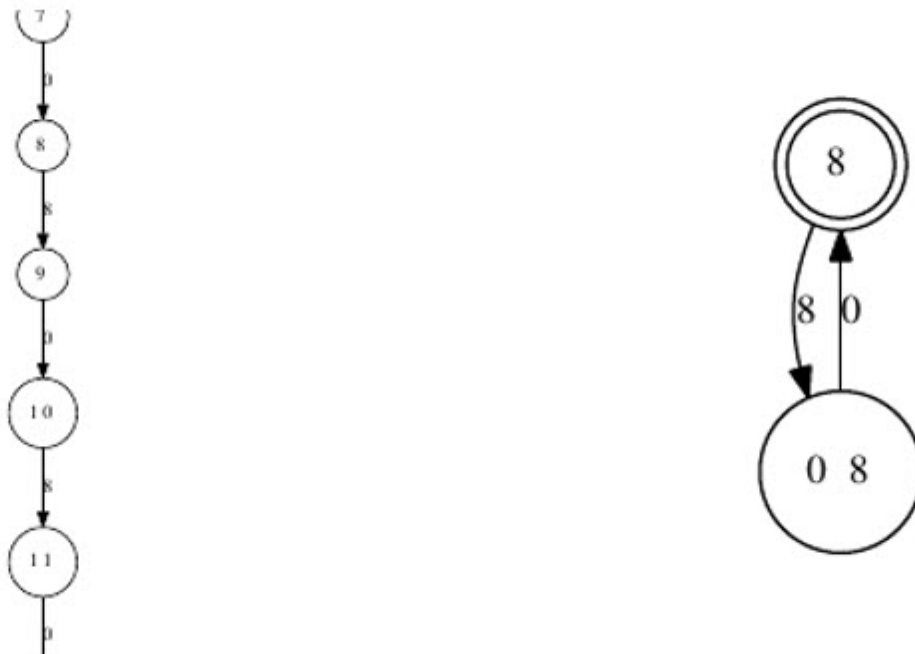
Fig. 5 State tree file output (left); final Ping protocol state machine (right)
