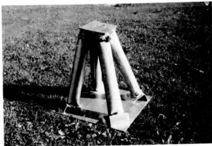
Figure 12 - Component Configuration with Four Energy-Absorbing Elements
