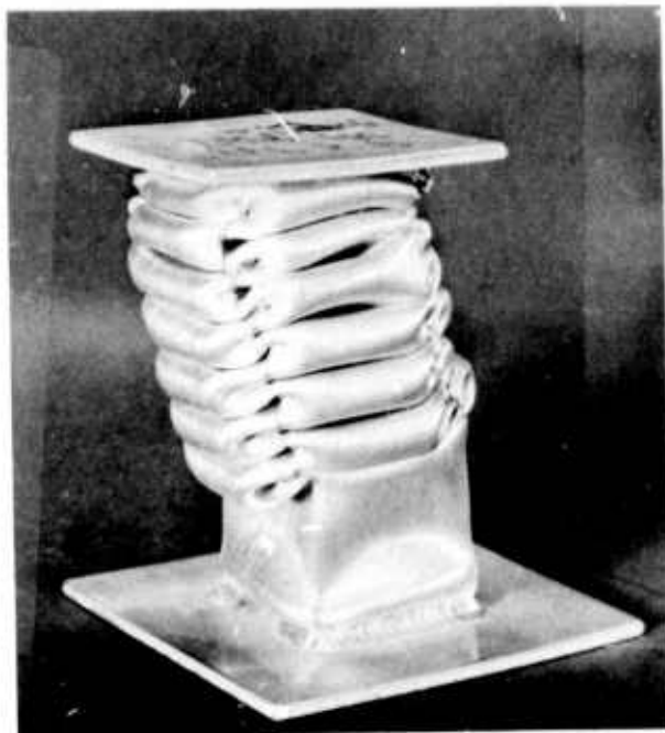
Figure 13 - Inextensional Buckling in a Square Tube
