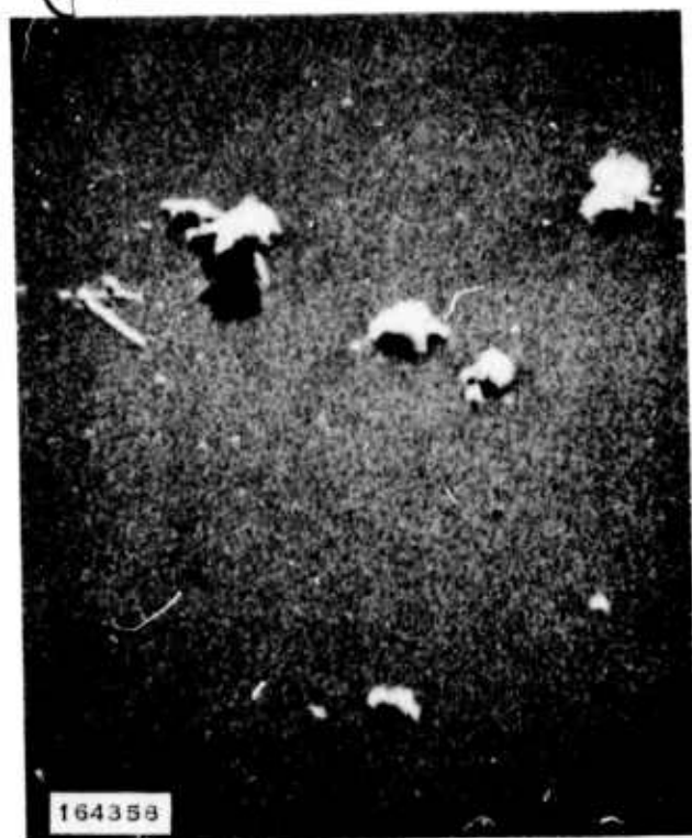
Figure 4-1. Particulate Contamination of a Si Slice after Storage for 2 Weeks in a Plastic Box (SEM Photograph; 20,000X)
