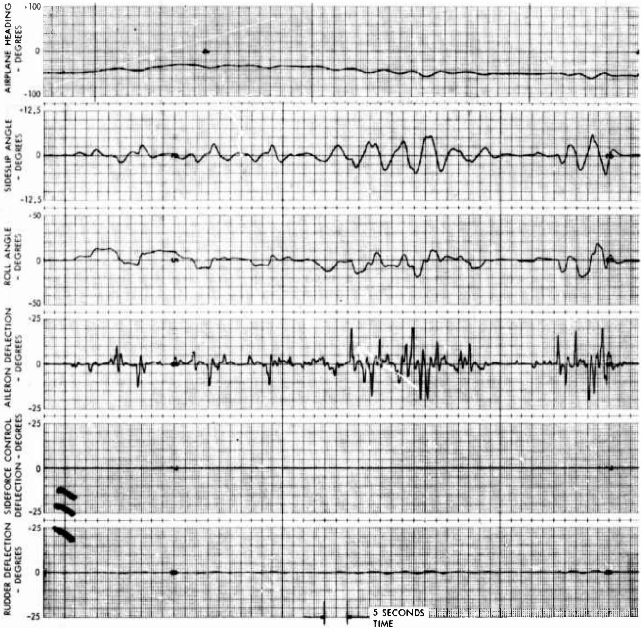
Figure J-5 Landing Approach with Zero Crosswind - Conventional Configuration
