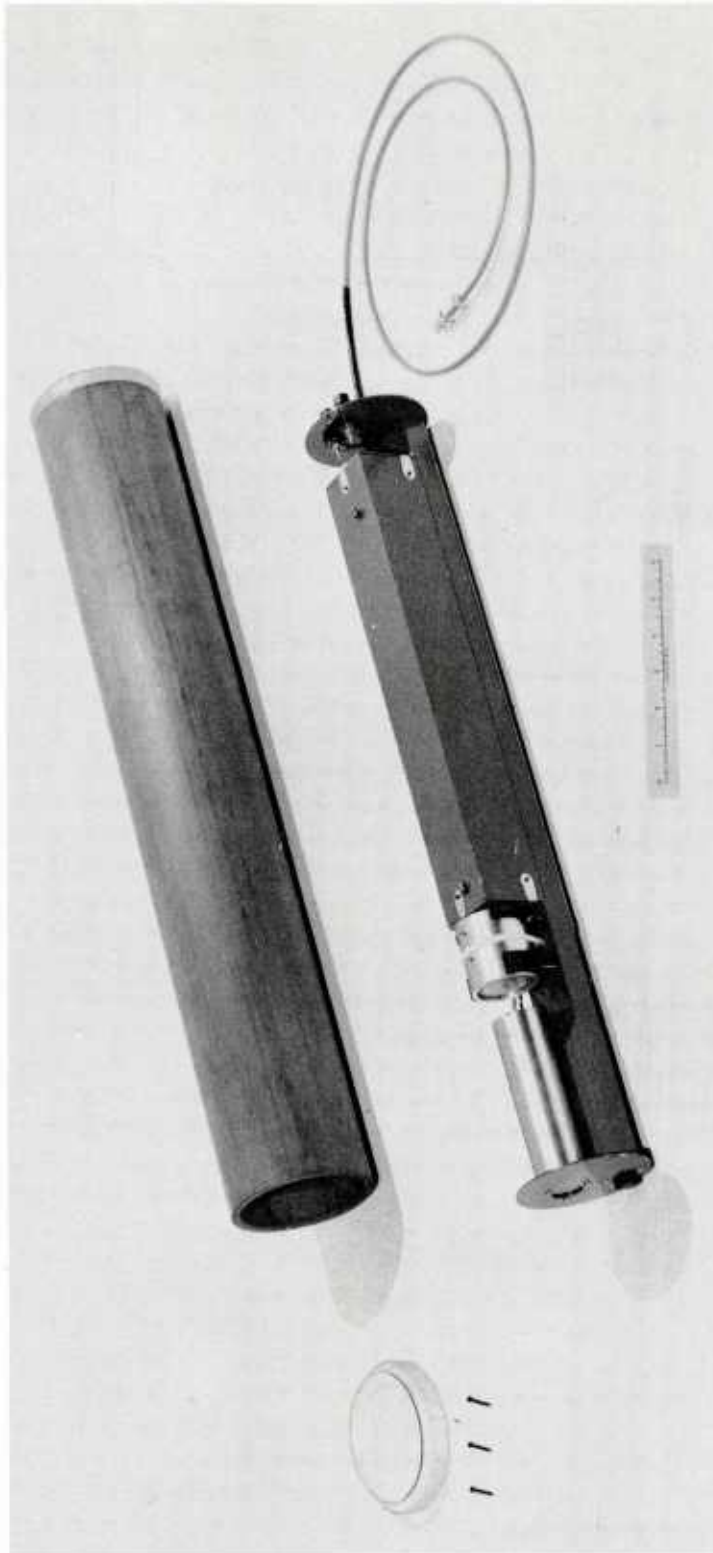
Figure 2.11 NUC polarization meter and waterproof polyvinyl chloride (PVC) housing.
