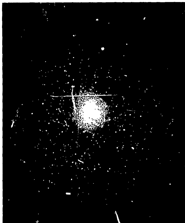
Figure 16 Scatter characteristics (magnification 28) of Lambda 3.5 micron doubly-resonant ZnS-ThF 4 mirror.
