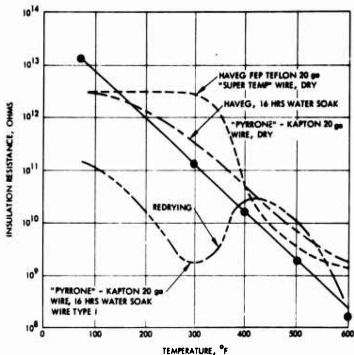
Figure 6. Effect of temperature on insulation resistance
