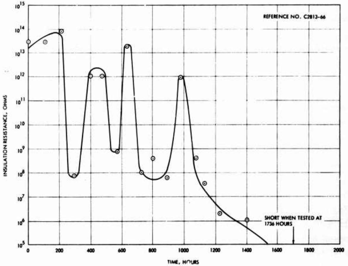
Figure 32. Insulation resistance as a function of thermal aging in air at 500°F - Wire type IIΔ
