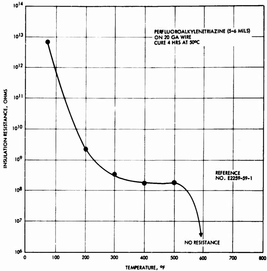
Figure 1. Insulation resistance of perfluoroalkylenetriazine insulated wire
