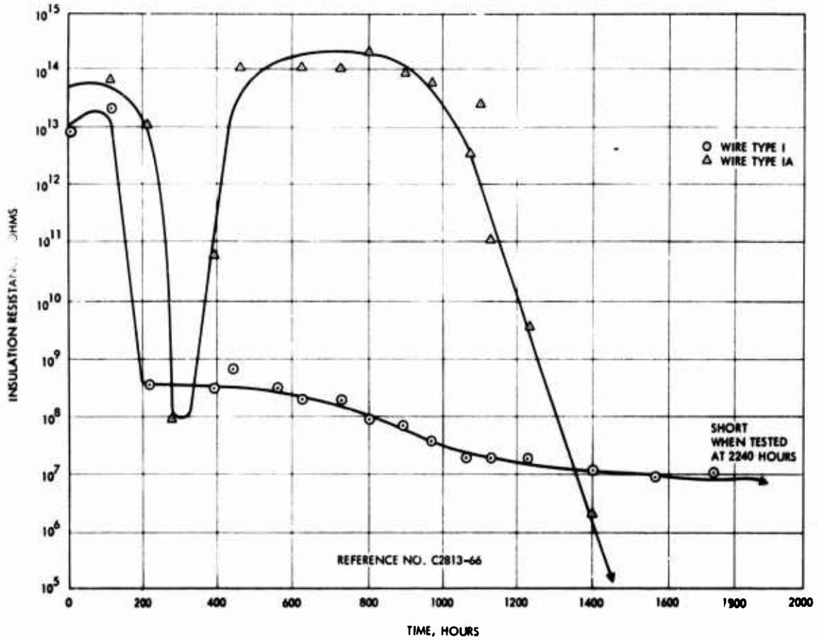
Figure 28. Insulation resistance as a function of thermal aging in air at 500°F - Wires type I and IA
