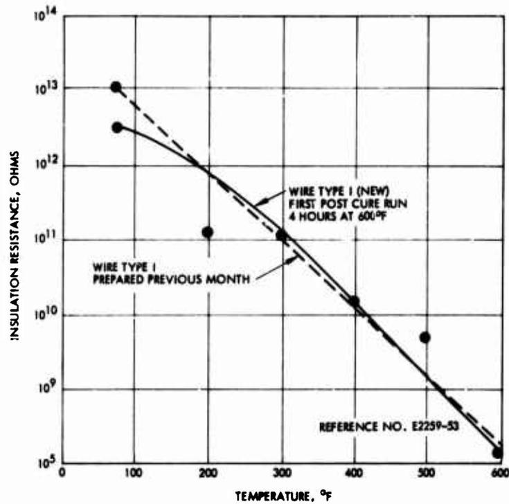
Figure 5. Insulation resistance of "pyrrone"-Kapton insulated wire
