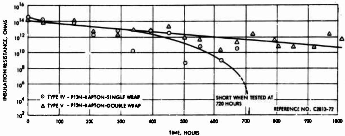
Figure 44. Insulation resistance as a function of thermal aging in air at 600°F – Wire types IV and V
