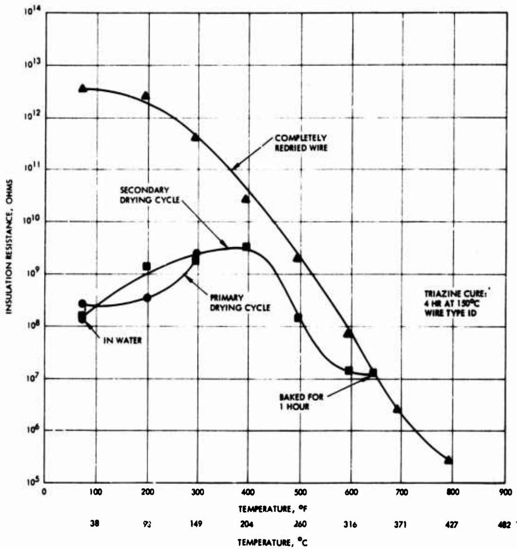
Figure 50. Insulation resistance as a function of temperature—perfluoroalkylenetriazine overcoated "pyrrone"-Kapton
