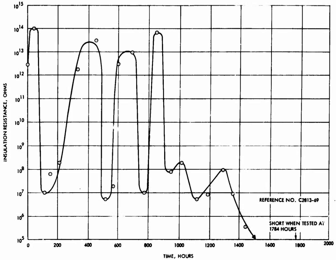
Figure 34. Insulation resistance as a function of thermal aging in air at  $550^{\circ}\text{F}$  - Wire type IA
