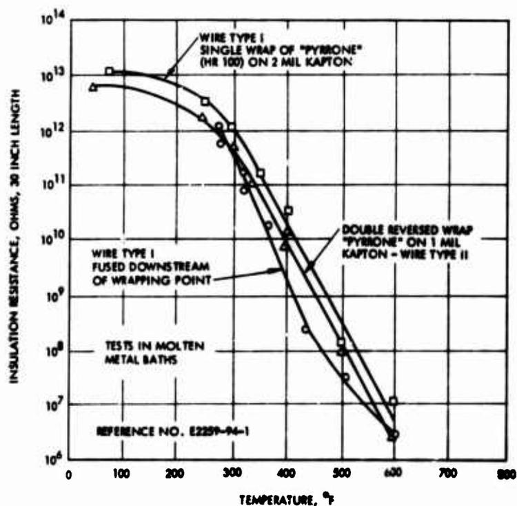
Figure 13. Insulation resistance of several "pyrrone"-Kapton insulated wires
