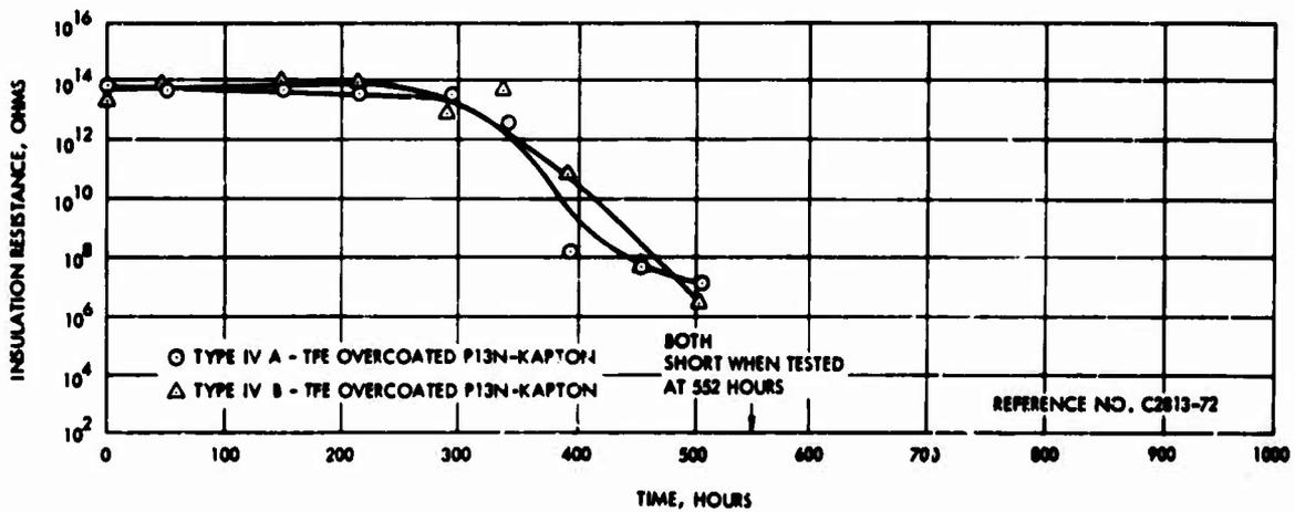
Figure 45. Insulation resistance as a function of thermal aging in air at 600°F – Wires type IVA and IVB
