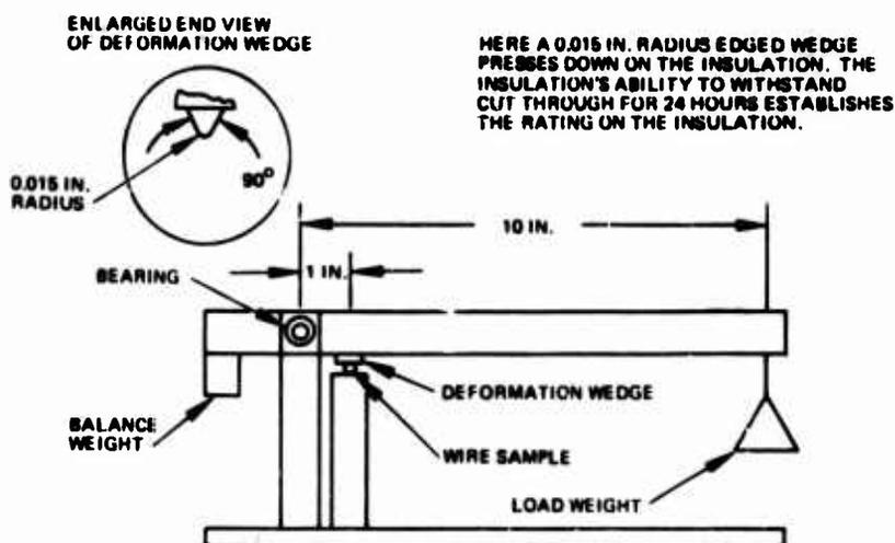
Figure 59. Insulation cut through tester
