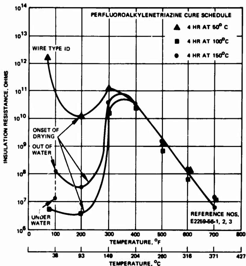
Figure 12. Insulation resistance of perfluoroalkylenetriazine coated "pyrrone"-Kapton insulated wire
