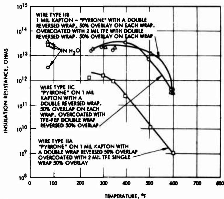
Figure 16. Insulation resistance of Teflon overcoated "pyrrone"-Kapton insulated wires as a function of temperature
