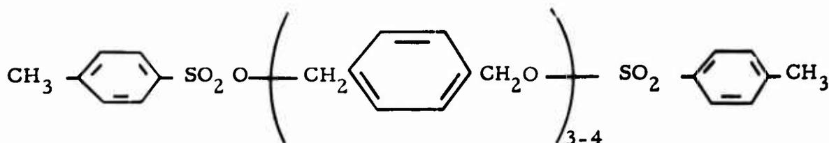
weight (based on solids) of the xylylene glycol telomer. Each of these mixed lacquers was used to bond together sheets of Kapton film and the laminates were cured for 1-1/2 hours at 750 psi and 250°C (482°F). Both of the laminates qualitatively exhibited peel strengths greater than that obtained from polyterphenyleneoxide alone. However, neither was sufficiently good to warrant quantitative tests.
