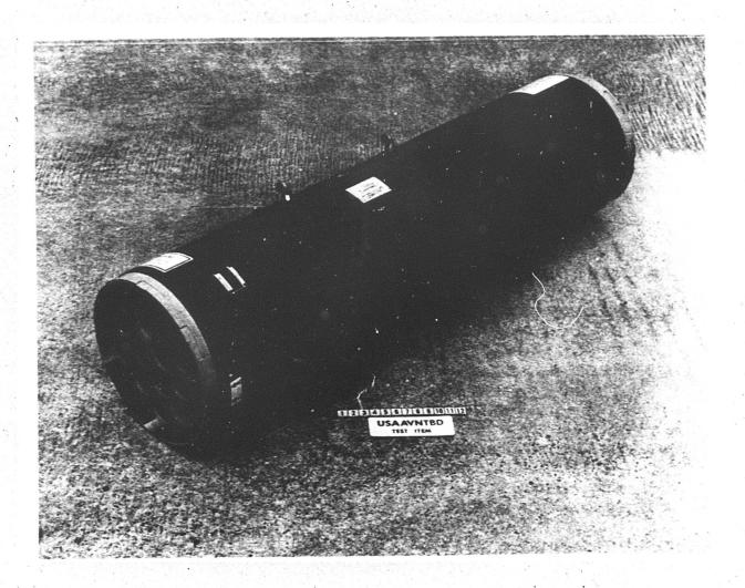
Figure 1. XM200 2.75-Inch Rocket Launcher
