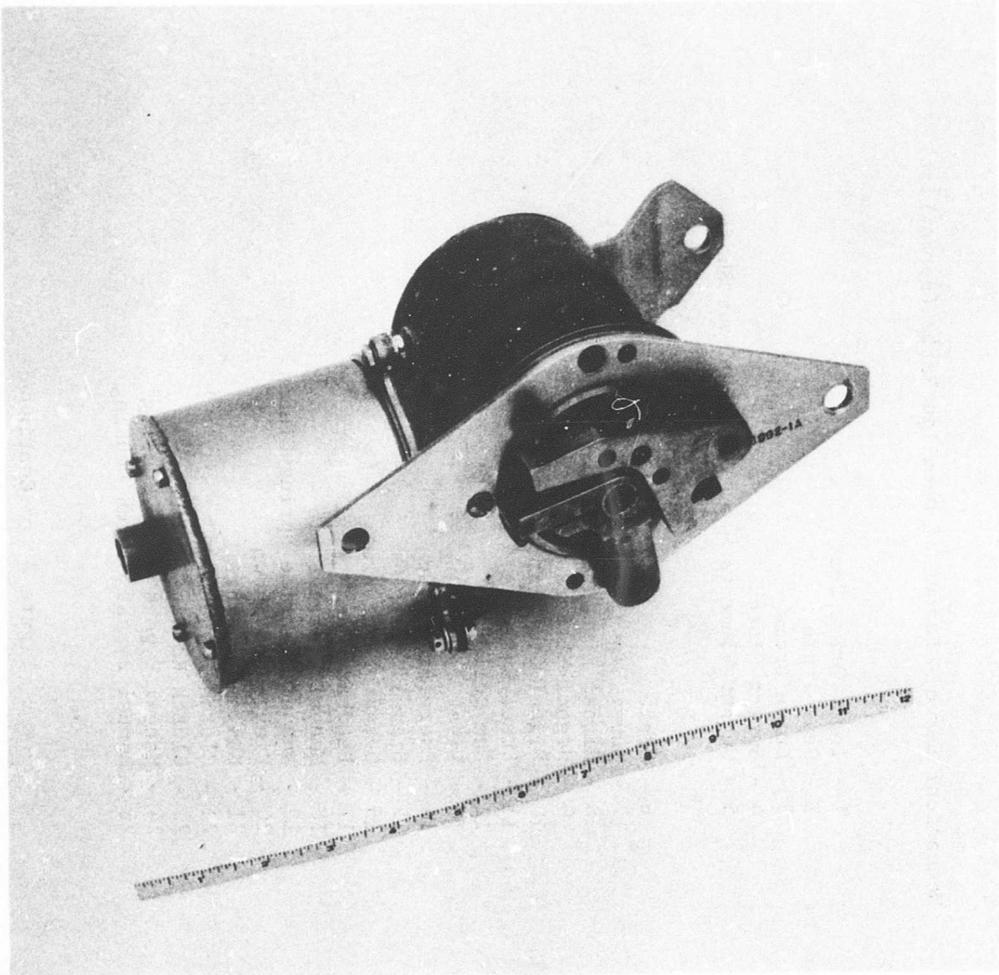
Figure 3. Mechanical Servo - Front View Assembly.
