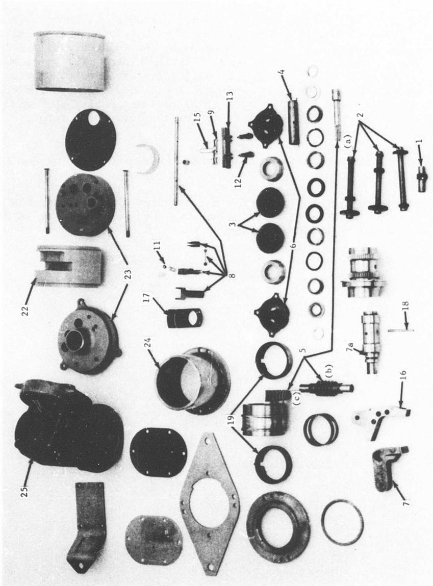
Figure 2. Mechanical Servo - Layout of Detailed Parts.
