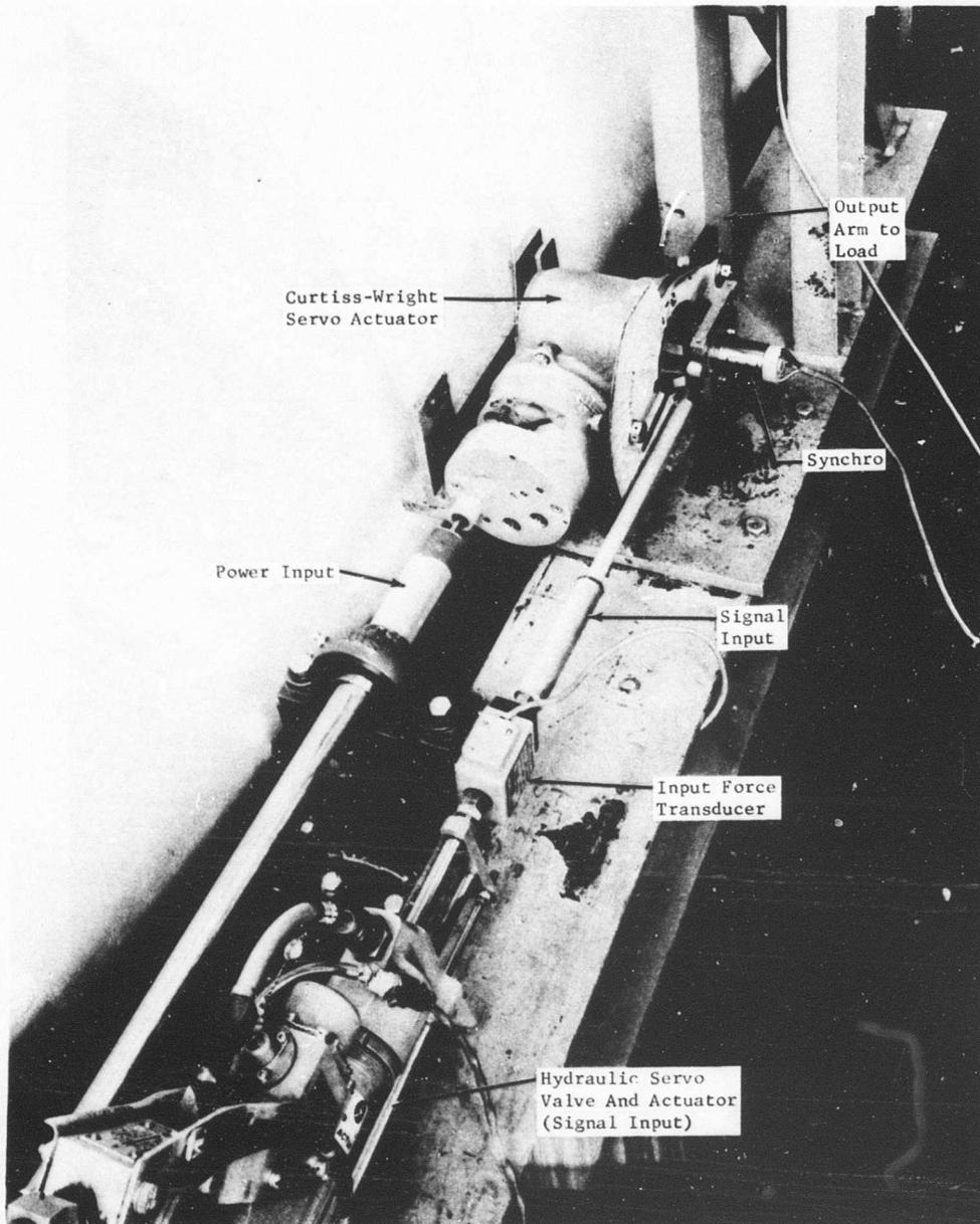
Figure 7. Mechanical Servo - Test Rig With Unit Installed.
