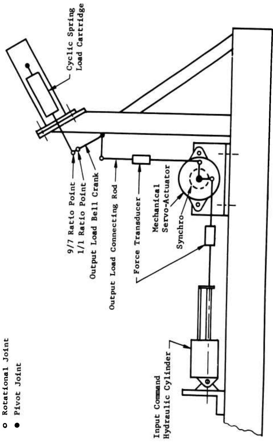
Figure 9. Schematic Diagram - Mechanical Servo-Actuator Installed on Test Fixture.
