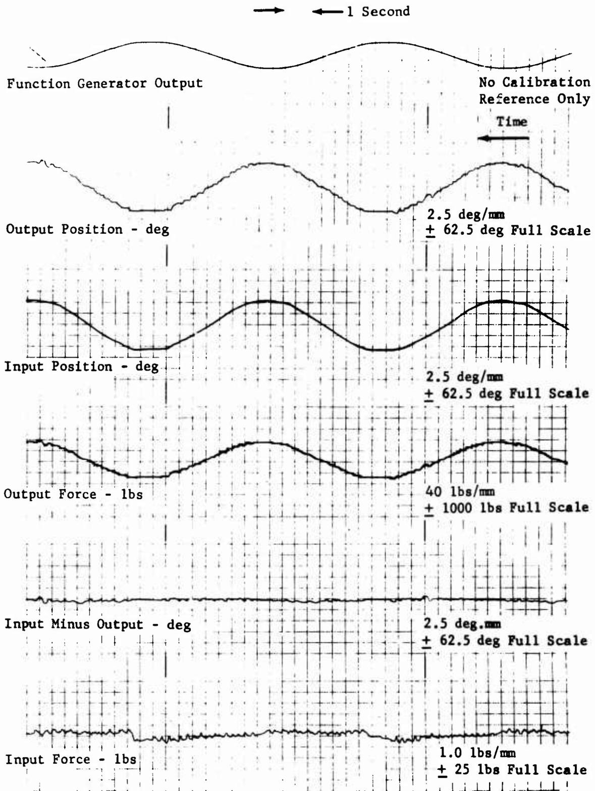
Figure 12. Endurance Cycling - Mechanical Actuator - 510-Pound Spring, 78-Percent Stroke, 0.1 cps.
