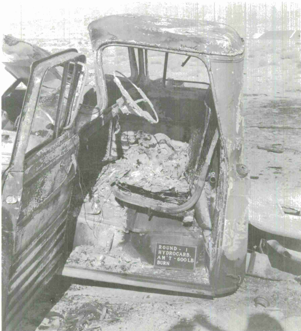
FIG. 4. Destruction of Mannequin and Cab Interior, Test 1.
