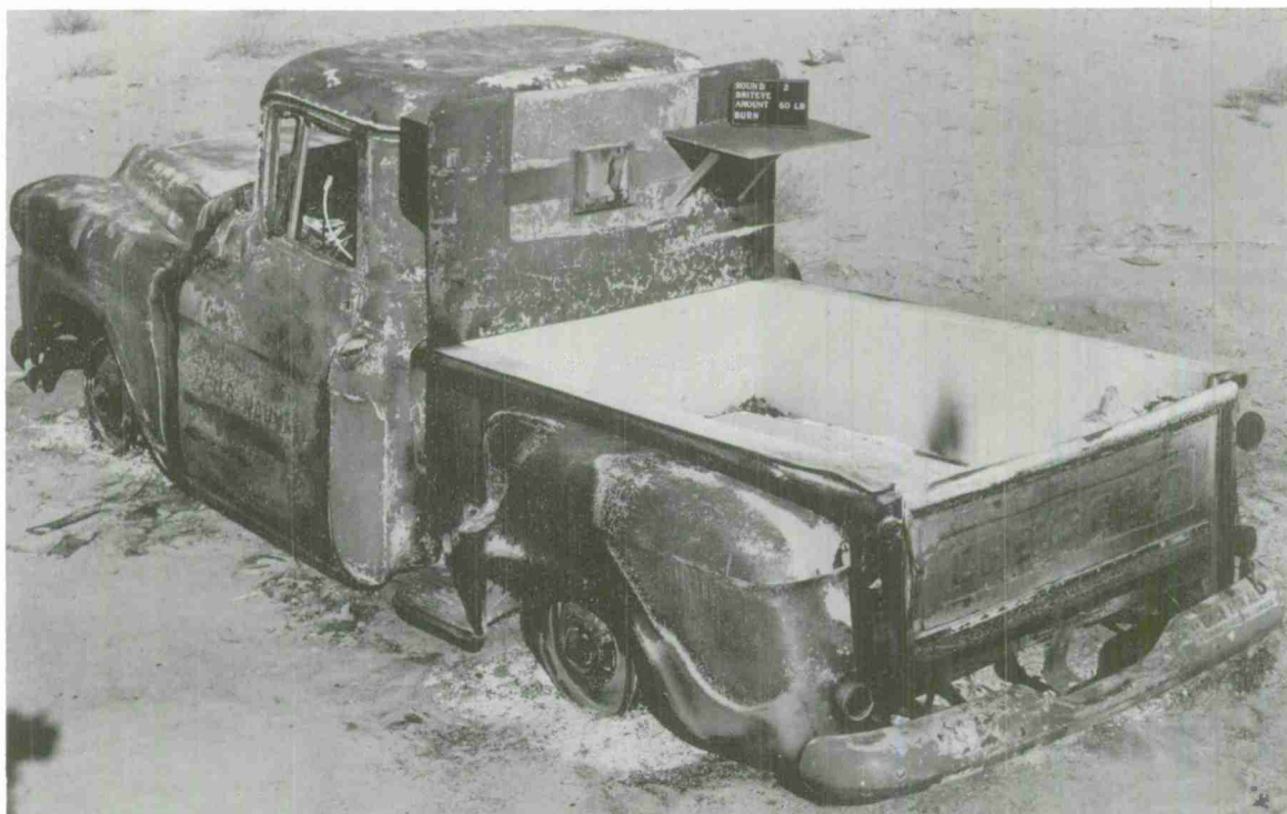
FIG. 6. Truck After Burning, Test 2.
