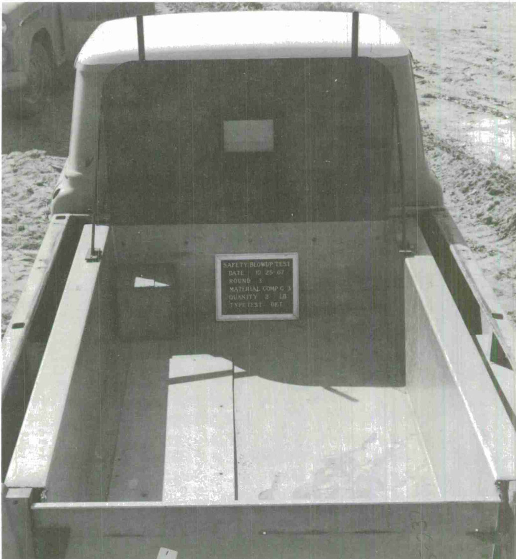
FIG. 9. Truck Bed With 2-Pound Block of Composition C-3 in Place for Test 3.
