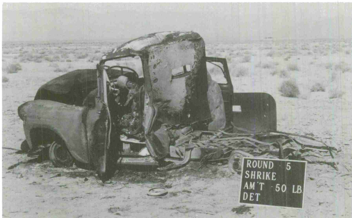
FIG. 18. Condition of Truck After Detonation of 50 Pounds of PBXC-104 Explosive, Test 5.
