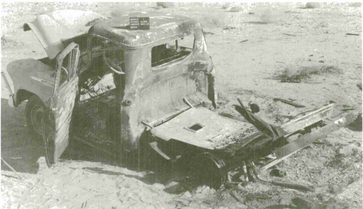
FIG. 3. Truck Damage From Burning and Subsequent Explosion of 600 Pounds of Propellant, Test 1.
