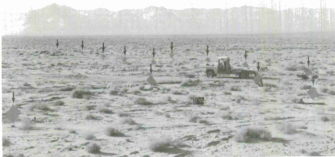
FIG. 16. Dispersion of Truck Fragments (Arrows), Test 4.
