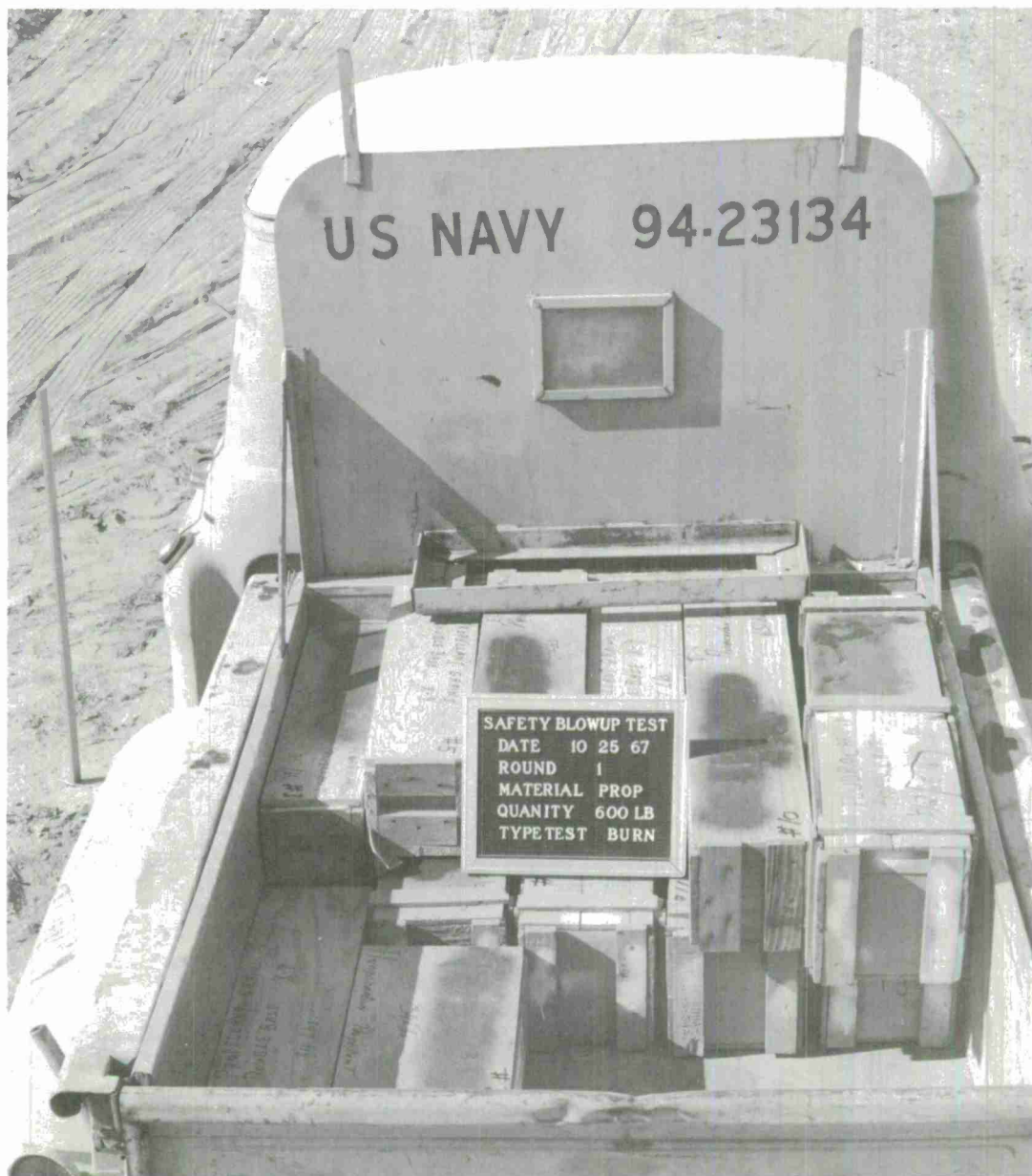
FIG. 2. Boxed Bulk Propellant Loaded on Truck Bed for Burning, Test 1.
