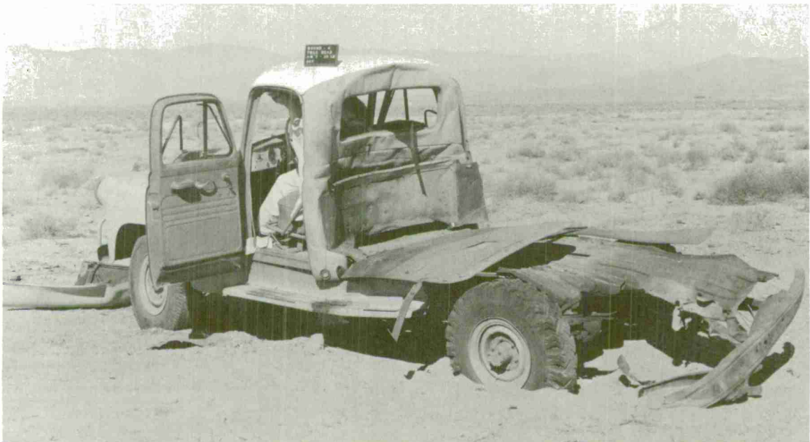
FIG. 14. Damage Resulting From Detonation, Test 4.
