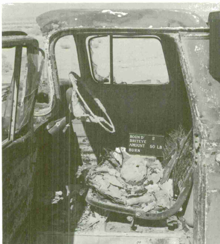
FIG. 8. Destruction Resulting From Reignition Caused by Residual Heat of Combustible Material, Test 2.
