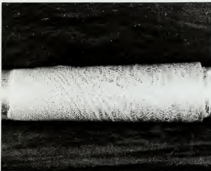
Fig. 18 The effects of humidity on Photostress Plastic in the curing stage.
