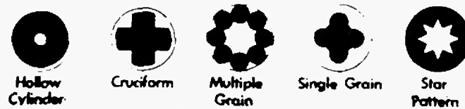
Fig. 2-6 Geometry of some rocket solid propellant charges.
