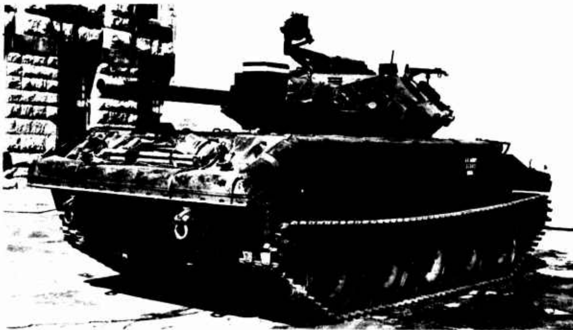
Figure 13 M103E7 105mm Cannon In M551 Vehicle
