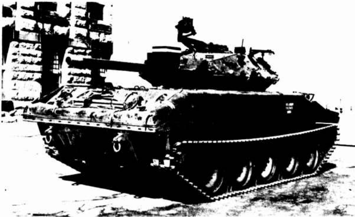
Figure 17 M103E7 105mm Cannon In M551 Vehicle
