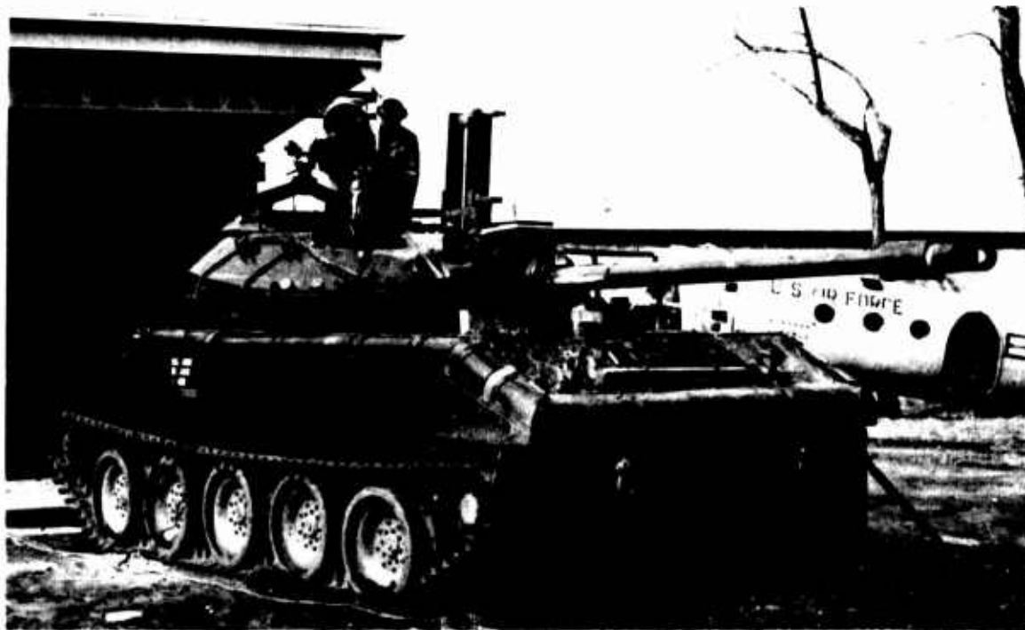
Figure 14 M32 76mm Cannon In M551 Vehicle
