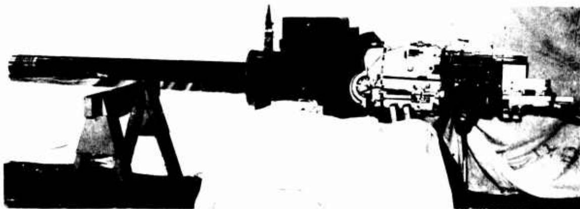
Figure 2 M103 Cannon Adapted to M81 Mount
