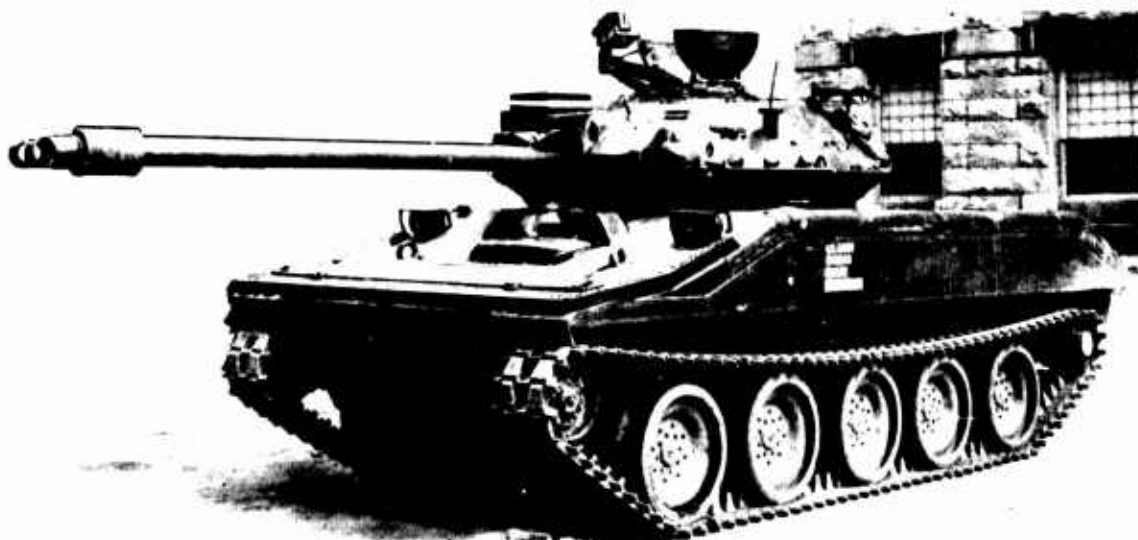
Figure 18 M76 Cannon & Mount In M551 Vehicle
