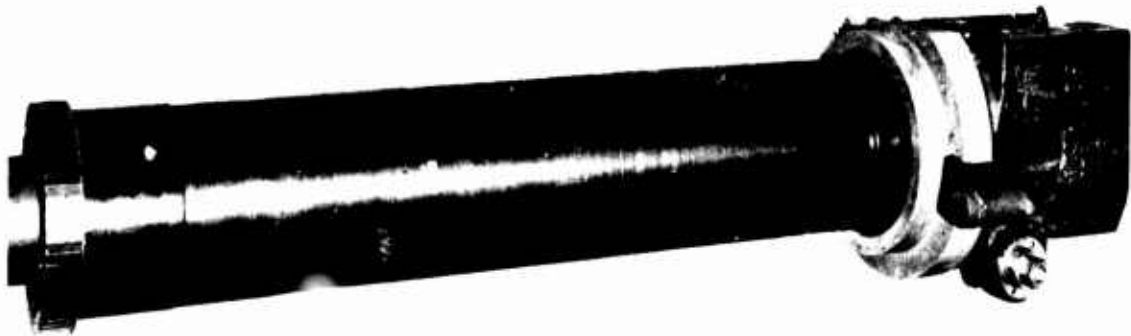
Figure 6 Adapter & Collar To Mate M32 Cannon With M551 Vehicle
