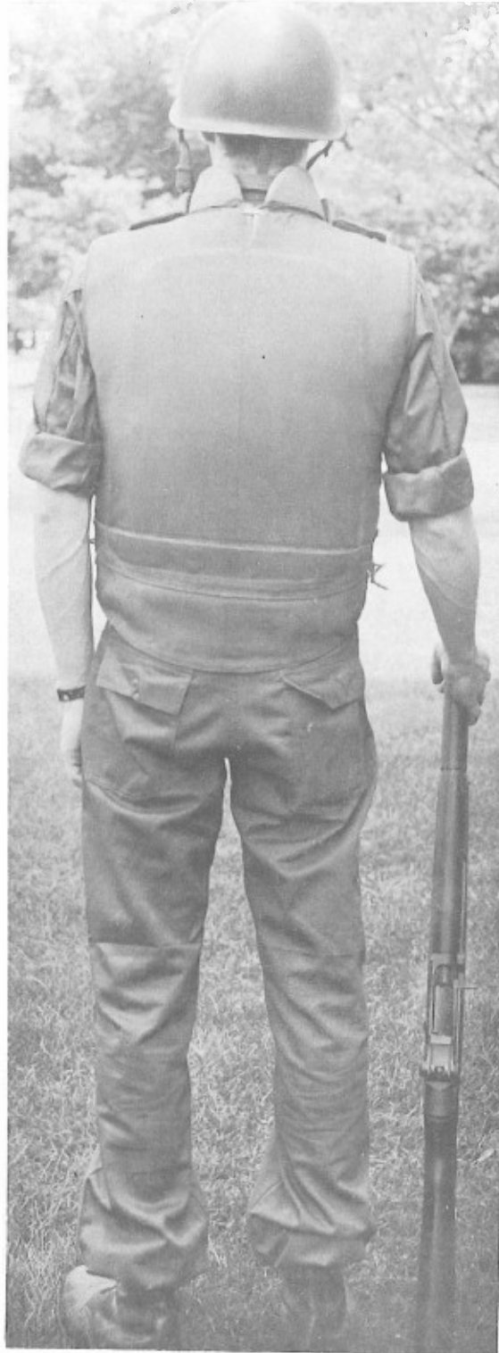
Figure 17. Model C, IITRI Integrated Jacket, Rigid Rear Element Retained in Integrated Pocket, Single Piece (Anatomically Contoured)
