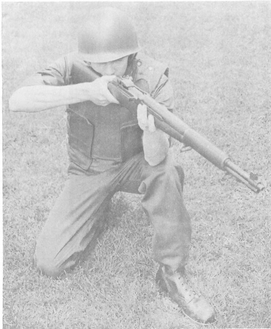
Figure 22. Model C, IITRI Integrated Vest, Kneeling Firing Position Note Articulation of Basic Garment at Waist
