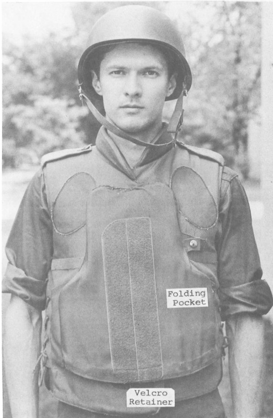
Figure 12. Model A, USANL Fragmentation Vest (Modified), Front Closure Showing Rigid Single-Piece Front Element Retained in Pocket (Anatomically Contoured)
