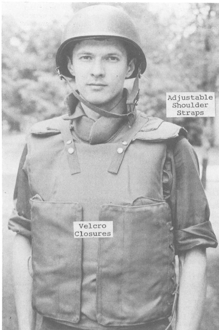
Figure 14. Model B, IITRI Jacket (Modified), Peripheral Protection Added, Overhead Donning, Rigid Articulated Front Elements
