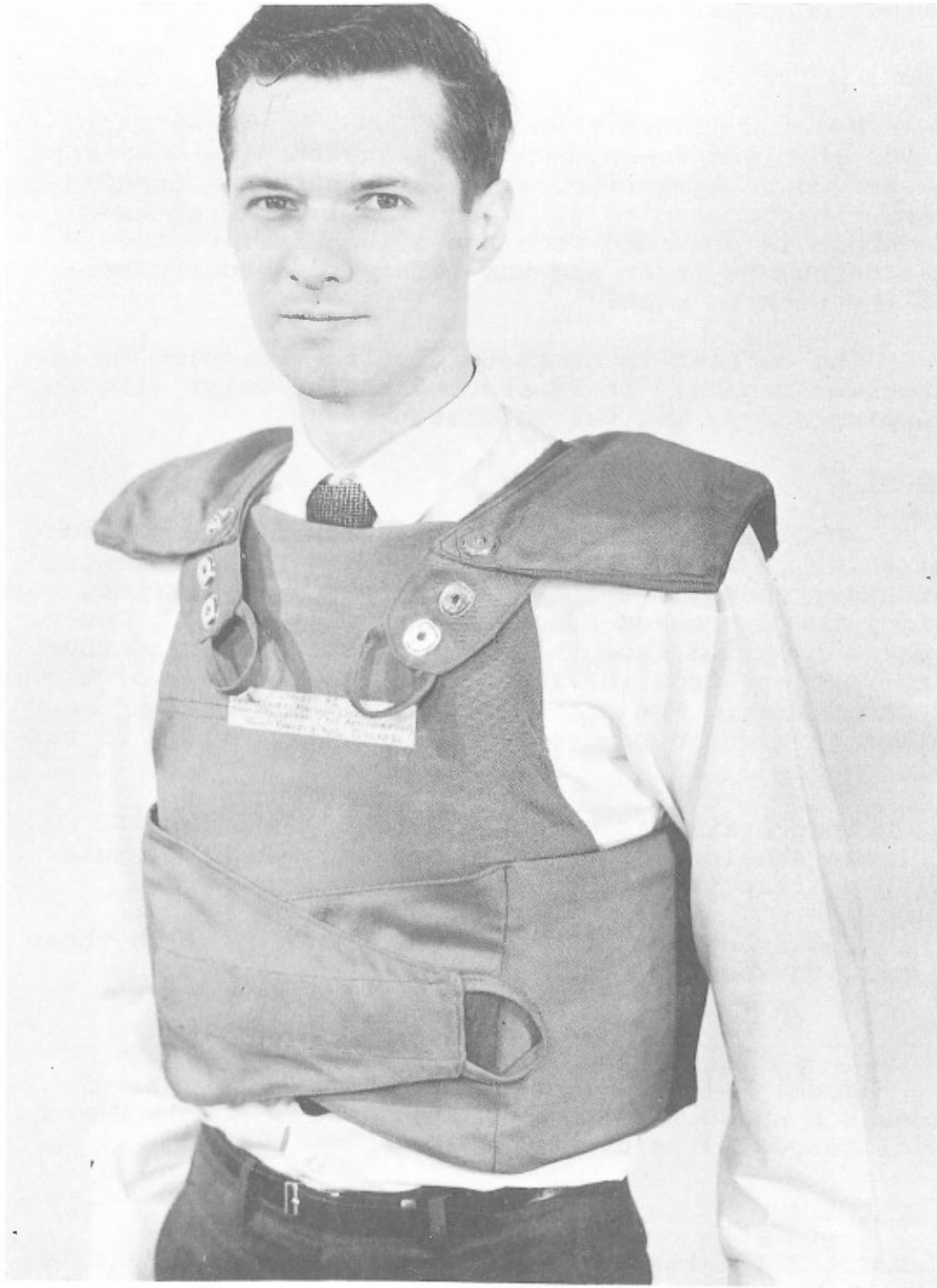
Figure 24. Model D, IITRI Rigid-Element Jacket, Nonarticulated, Overhead Donning
