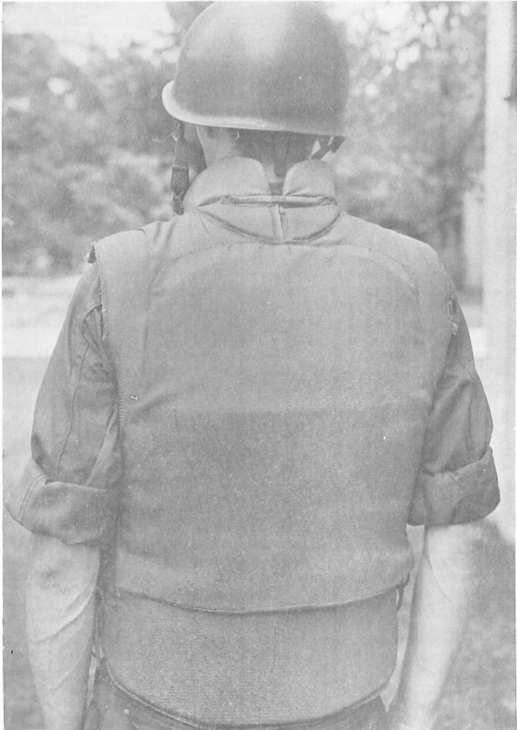
Figure 15. Model B, IITRI Jacket (Modified), Rigid Articulated Rear Elements Retained in Pocket (Anatomically Contoured)
