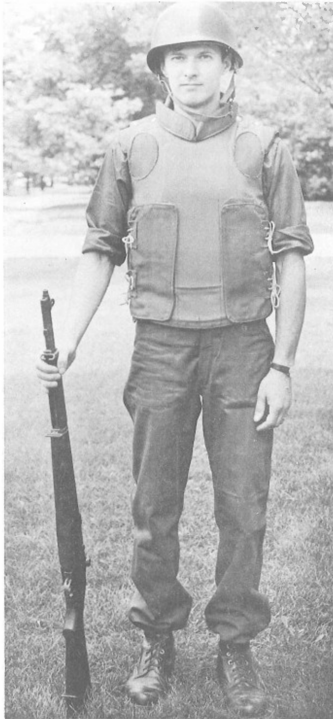
Figure 18. Model C, IITRI Integrated Jacket, Reduced Area Coverage, Front Element Permits Shouldering of Rifle
