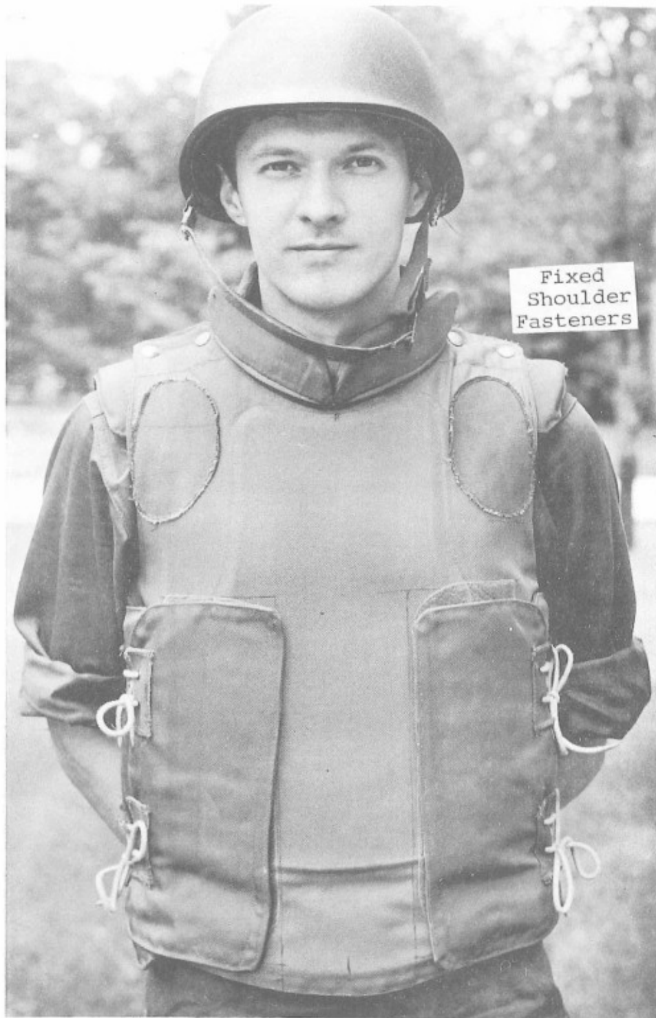
Figure 16. Model C, IITRI Integrated Jacket, Removable Single-Piece Front and Rear Elements, Side Closure, Overhead Donning
