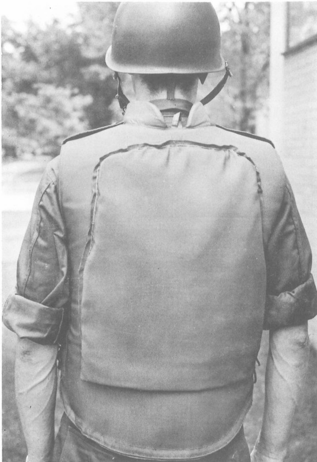
Figure 13. Model A, USANL Fragmentation Vest (Modified), Rigid Single-Piece Rear Element Retained in Pocket (Anatomically Contoured)
